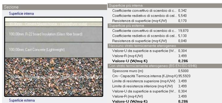
Figura 5 - Basamento in calcestruzzo su terreno, composto da: ceramic, glazed (2cm), cement screed (3 cm), R-22 board Insulation (glass fiber board) (10 cm), cast concrete (lightweight) (10 cm), miscellaneous materials, aggregate (sand/gravel/stone) (25 cm)
