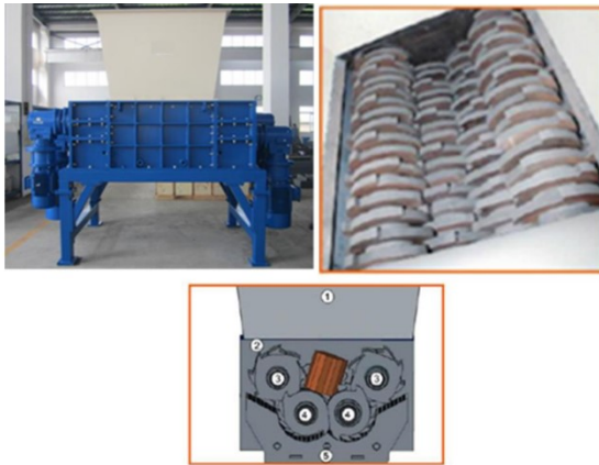
Figura 18 - Four shaft rotor shear [56].
