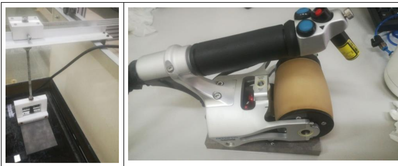
Fig. 11 setup semiautomatici con sonda phased array e Rollerform
