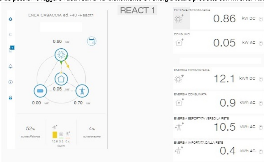
Figura 29. Misure inverter ABB REACT1
