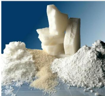
RUBITHERM® RT is a pure PCM, this heat storage material utilising the processes of phase change between solid and liquid (melting and congealing) to store and release large quantities of thermal energy at nearly constant temperature. The RUBITHERM® phase change materials (PCM's) provide a very effective means for storing heat and cold, even when limited volumes and low differences in operating temperature are applicable.
