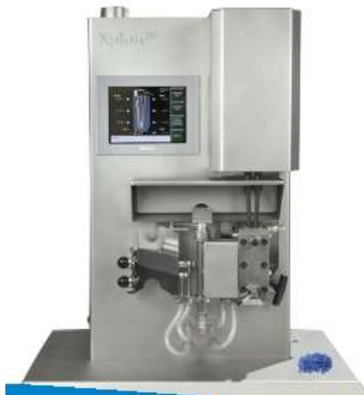
Figura 8. DSM Xplore 5 ml Micro-compounder (NL)
