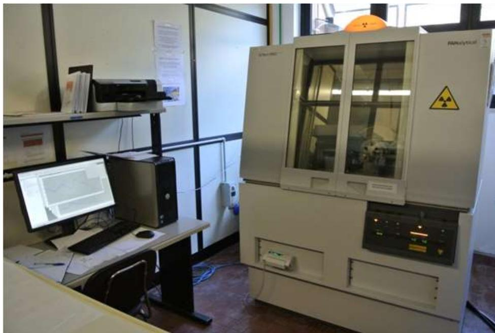
**Figura 28. Diffrattometro PANalytical X'Pert PRO**
