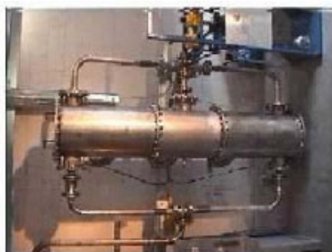
Figura 9: Reverse Flow Tar Converter [5].
