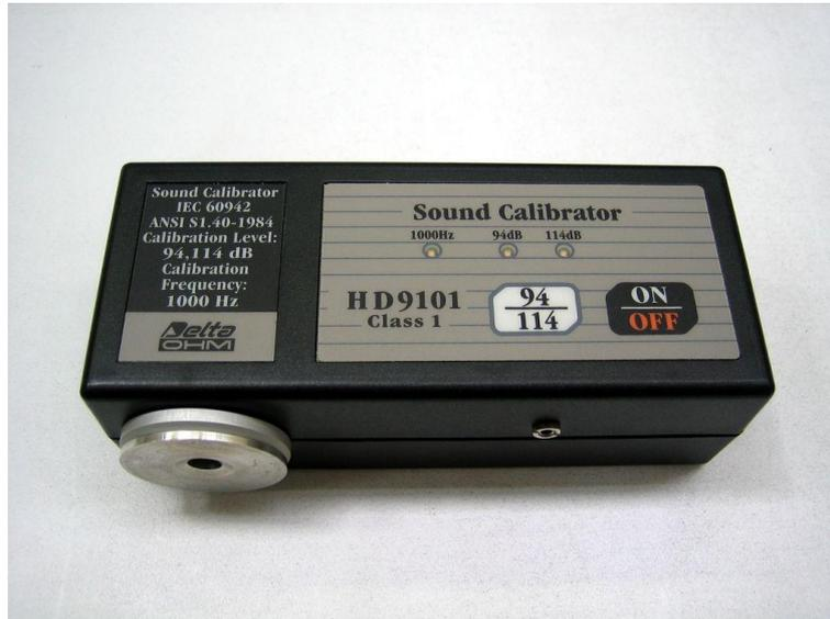
Figura 2.15: calibratore “Delta Ohm Sound Calibrator HD9101 class 1”.
