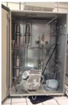
Figure 2. Pictures of membrane gas permeation test rig for single/mixed gas(left), membrane permeation test rig for humidified conditions(middle) and membrane permeation test rig for mixed gas at high pressures (right)
