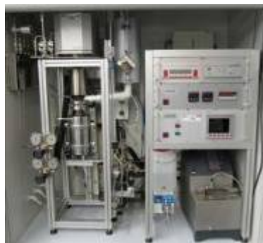
Magnetic suspension balance equipped with steam generation and multiple gas inlet systems.
