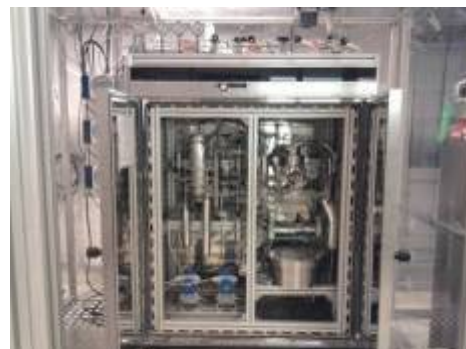
Figure 2. Pictures of membrane gas permeation test rig for single/mixed gas(left), membrane permeation test rig for humidified conditions(middle) and membrane permeation test rig for mixed gas at high pressures (right)
