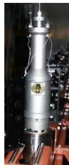
Fig. 4: Fluid cell for IFT-measurements (working conditions: 700 bars and 180 °C)
