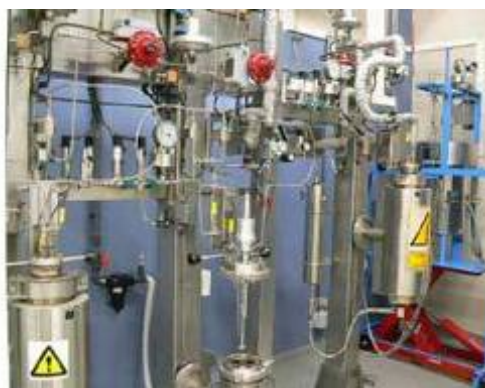
Equipment available in the High Pressure lab: 300 ml reactor (left), pilot plant equipped with 16 litres high pressure vessel (center) and SCF View Cell Thar (Right).
