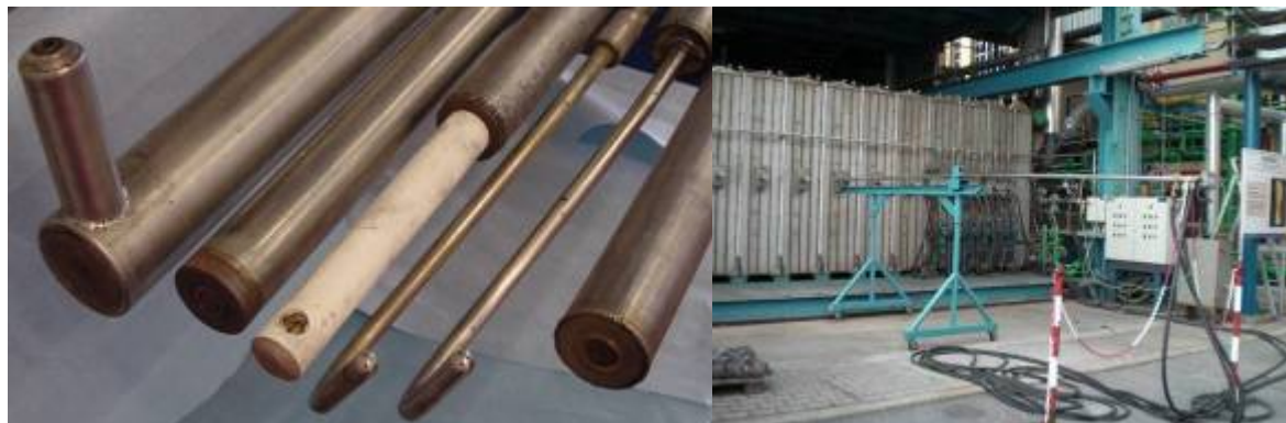
IFRF probes for in-flame measurements in FO.SPER
