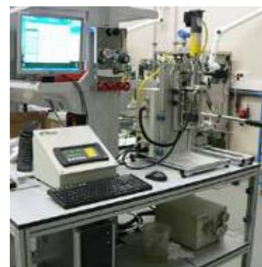
Equipment available in the High Pressure lab: 300 ml reactor (left), pilot plant equipped with 16 litres high pressure vessel (center) and SCF View Cell Thar (Right).
