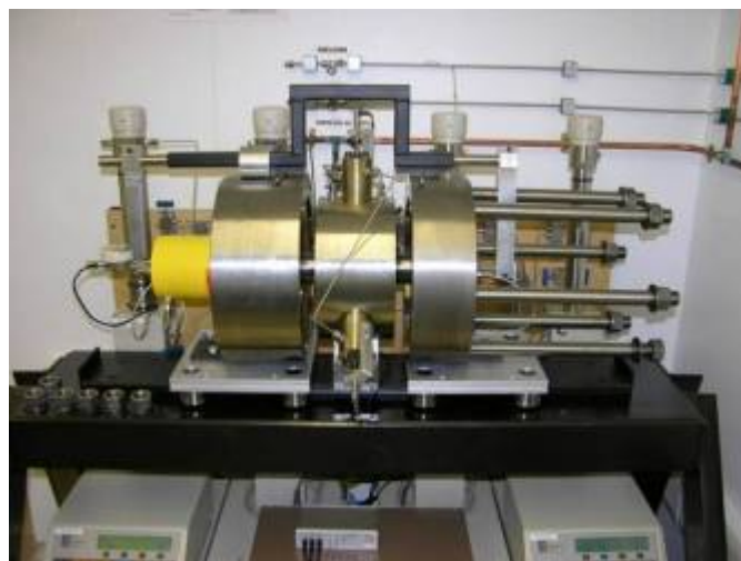
Intrinsic permeability measurement in the TPRL
