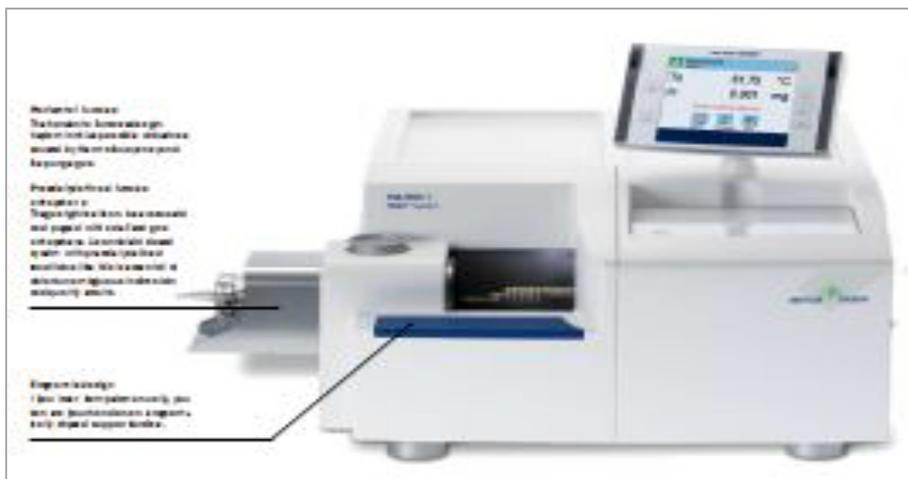
*Figura 1.2: Mettler-Toledo TG/DSC1 Star System*
