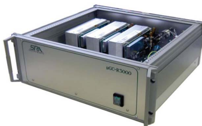
Figura 2.10. Micro gascromatografo SRA Instruments R-3000 Rack 19-inch.
