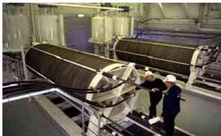
Norsk Hydro Electrolysers (485 Nm<sup>3</sup>/h)
