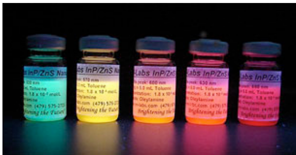
Fig.3 InP/ZnS quantum dots with different diameters – the right most QD’s are the ones used in this work.
