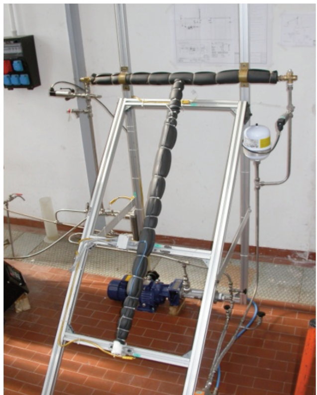
Impianto T.O.S.C.A. (Thermal fluid-dynamics Of Solar Cooling Apparatus)
