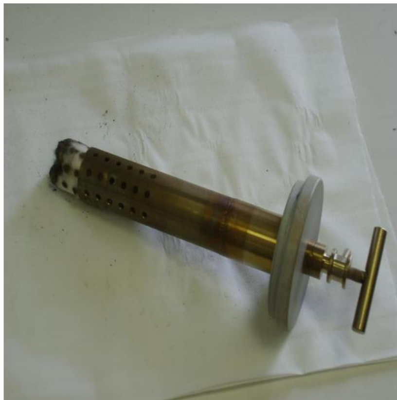
Figure 2. Photograph of filter of sampling probe after runs
