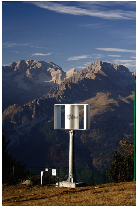
Figure 7 – A Ropatec small-sized vertical-axis turbine on Monte Casale in the Italian Alps near Trento (courtesy of Ropatec)
