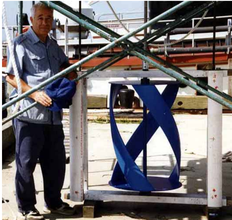
Figura 17. Turbina elicoidale Gorlov ( http://www.gcktechnology.com/GCK/pg1.html ).
