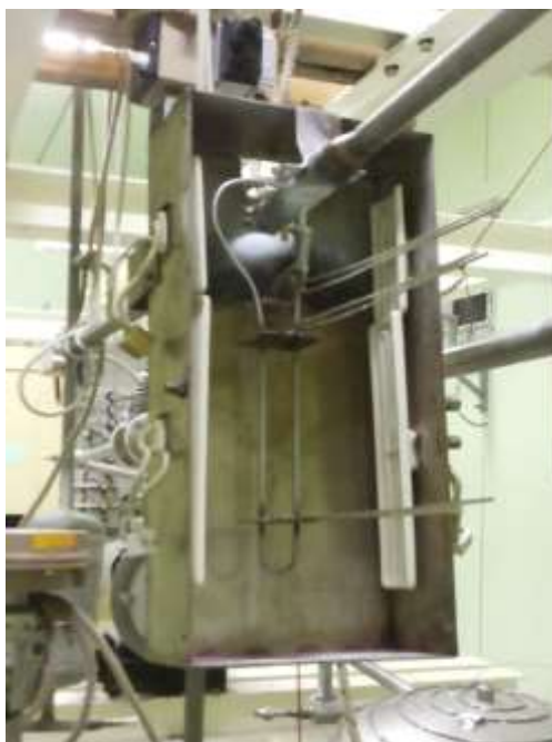
Figure 8 - R-meter installation on the purification branch
