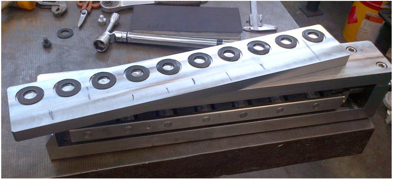
fig. 20 frame mock-up with Belleville springs
