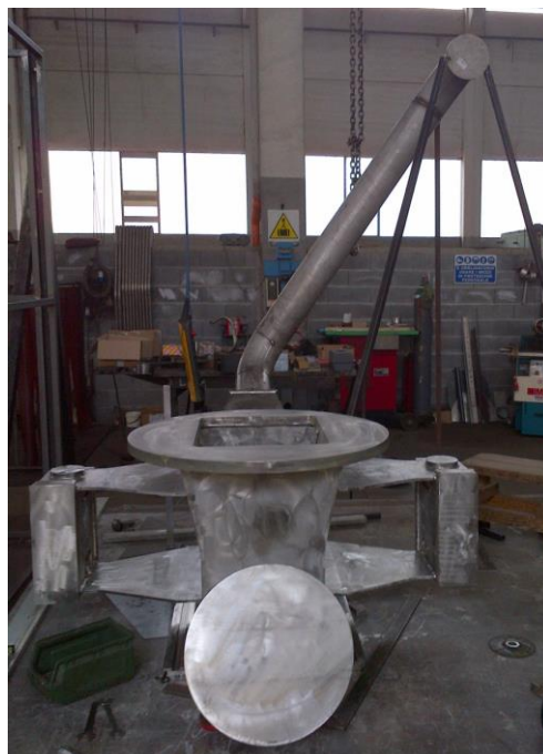
fig. 14 TA body welding (inlet pipe positioning)
