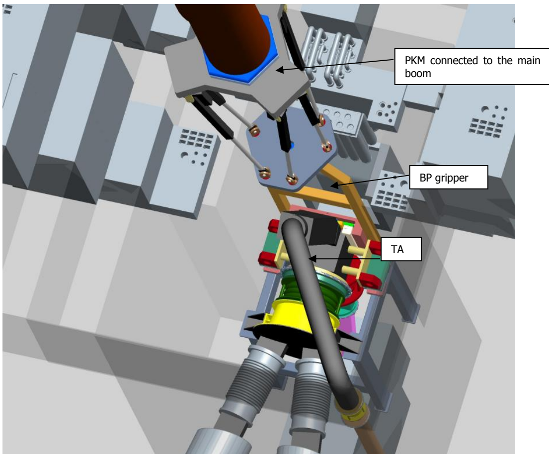
Fig. 2.21 - BP removal in Test Cell
