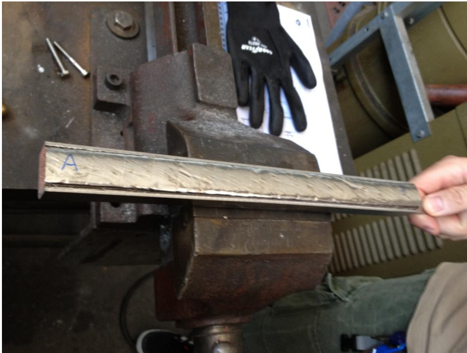
Fig. 4 He inlet insert welding sample before cable extraction
