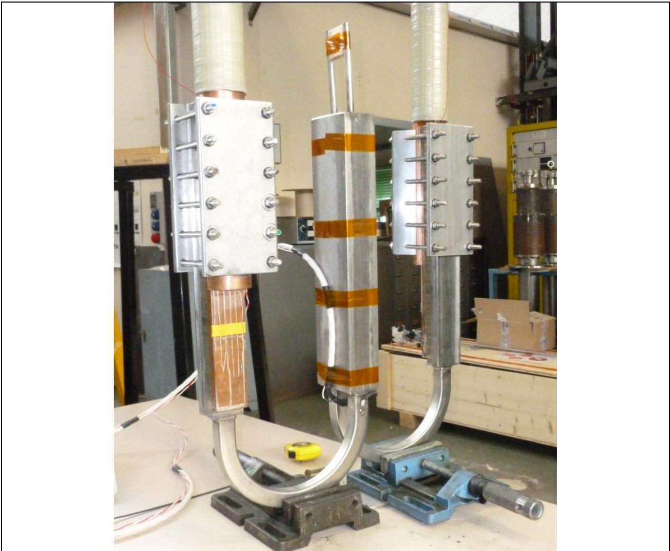
Figure 1: The connection among the copper terminations and the current leads has been realized by means of aluminium shoes, with the interpositions of indium wires on the contact surface.
