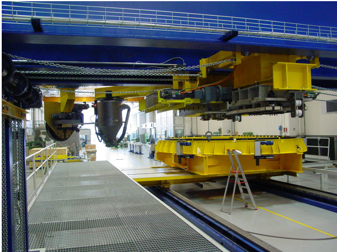
Figure 4 Driving carriage, bending unit, sand-blasting and taping machines mounted on the second portal.
