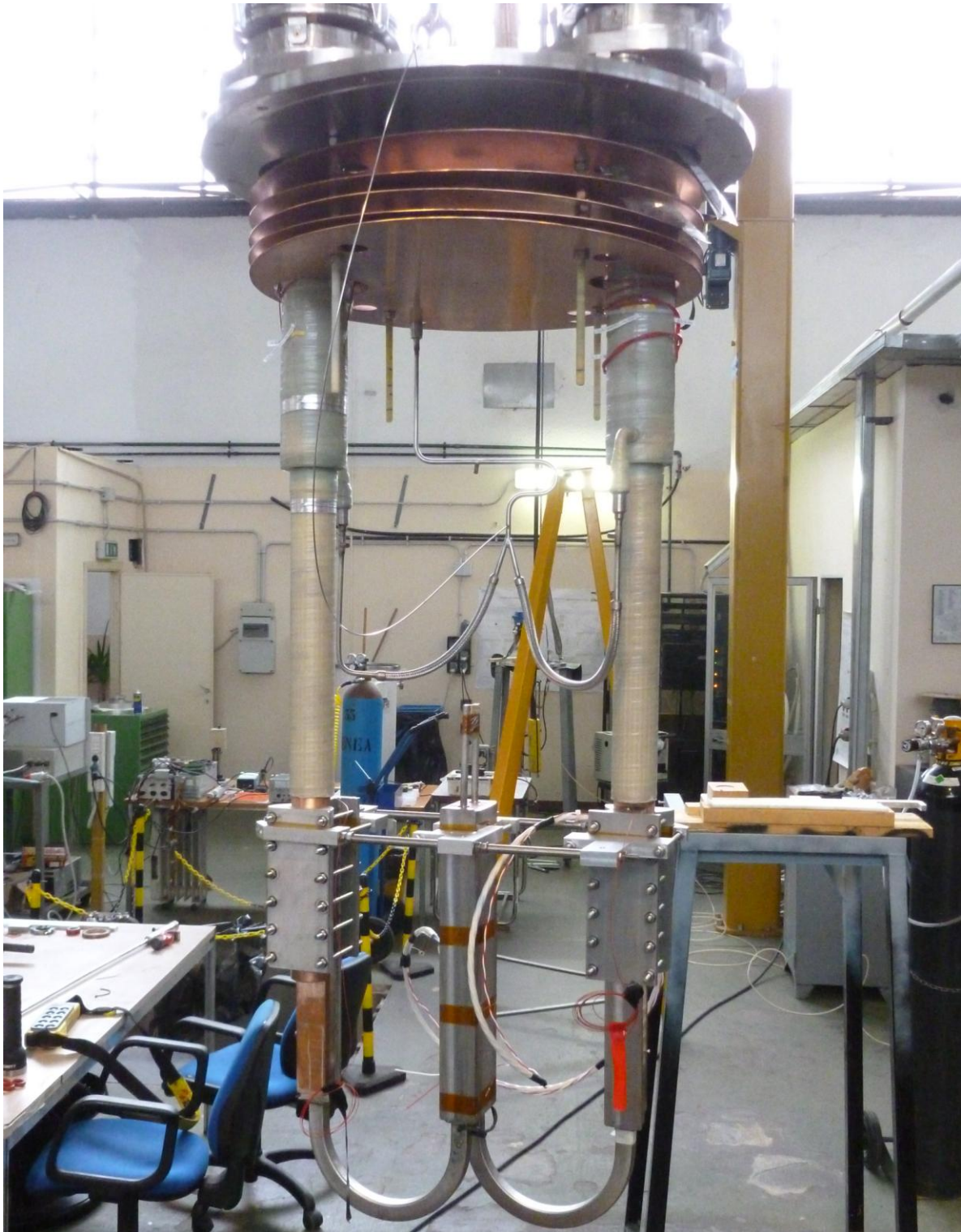
Figure 26 Electrical inner joint and termination mock-up before immersion in liquid He bath for electrical tests.
