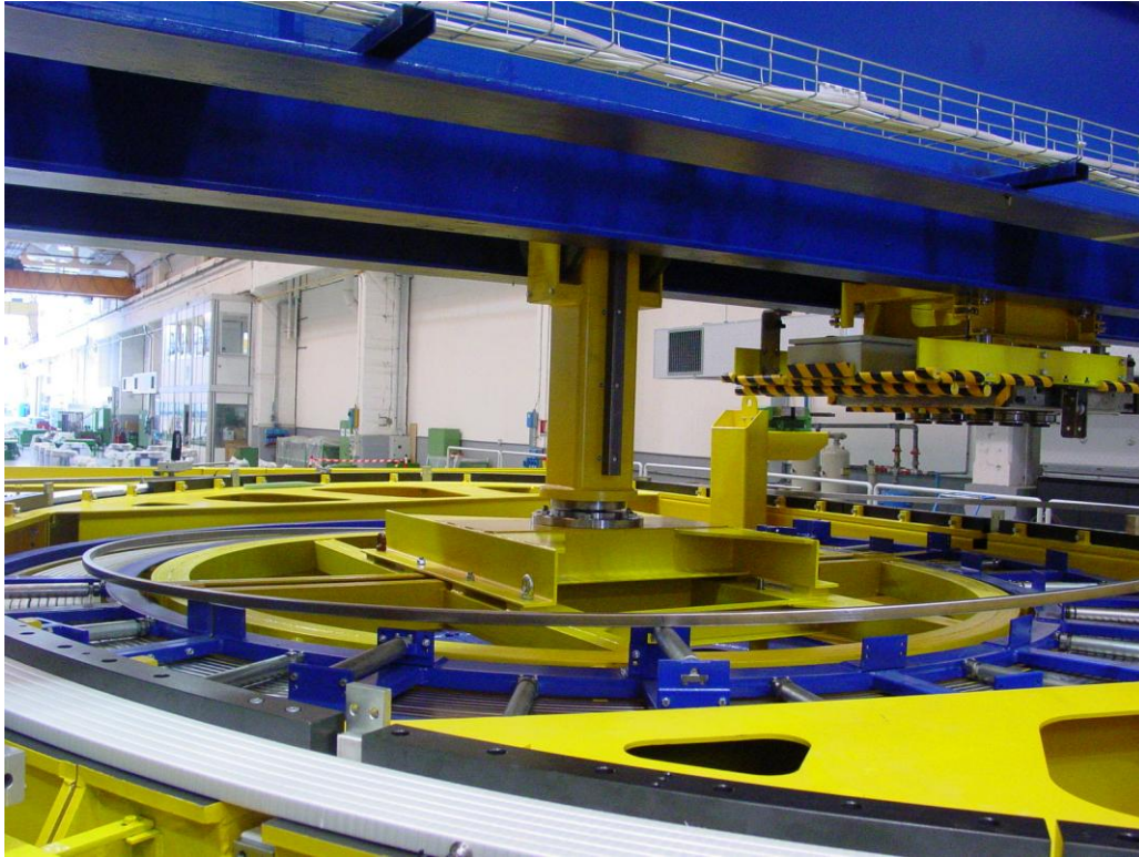
Figure 6 The reserve spool is picked up by the second portal and lifted from the roto-translating moving carriage.
