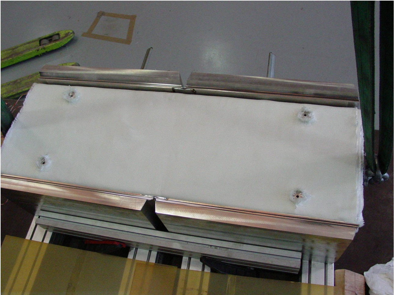
Figure 21 Insertion of impregnation beam and combination of the two halves of casing curved leg mock-up
