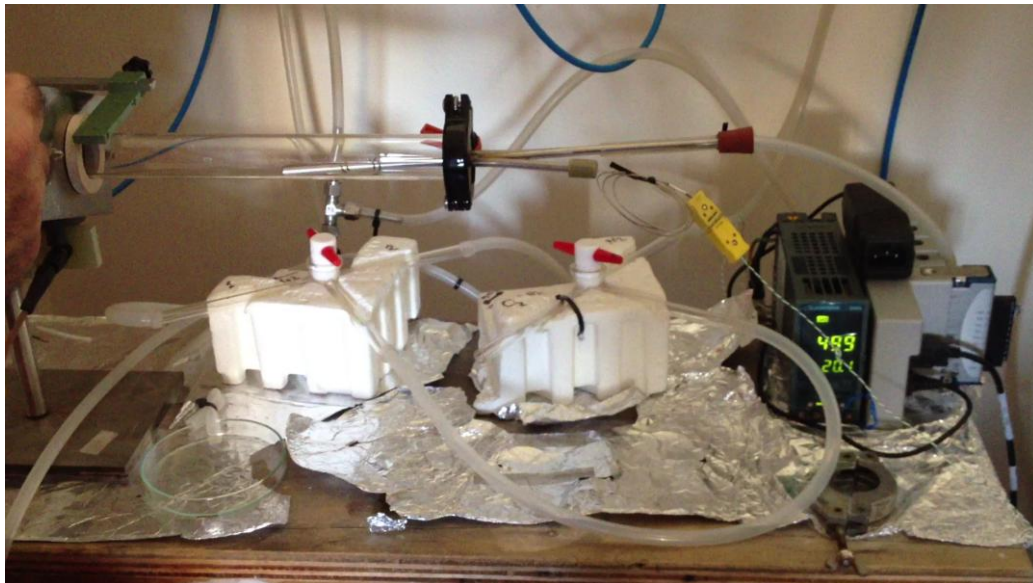
Fig. 8 Apparatus used to heat the strand samples up to 500 °C for 30 s.
