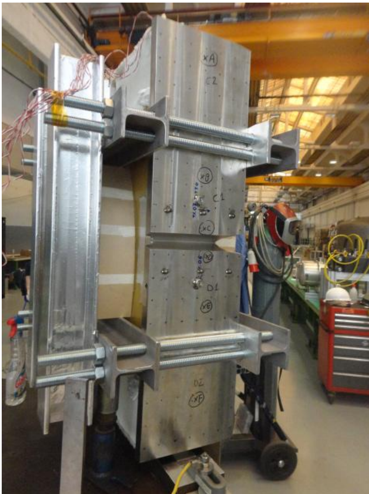
Figure 22 Transverse weld qualification on casing mock-up in the vertical position to simulate the operational conditions in the actual coil.
