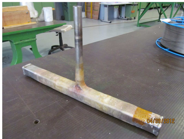
Fig. 12 – Campione He-inlet isolato / He-inlet insulation sample
