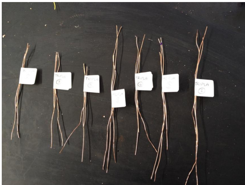
Fig. 7 Triplets extracted from cable after identification of possible damage.
