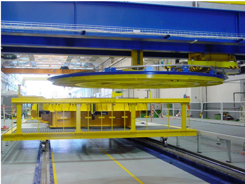
Figure 7 The reserve spool is rotated while the roto-translating moving carriage is moved away.
