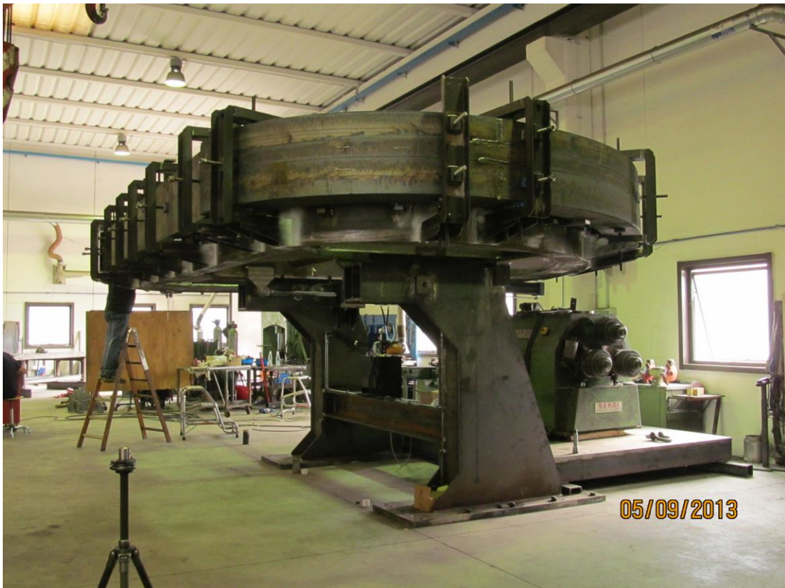
Figure 17 Tooling for WP into casing insertion rotated horizontal position to simulate the latest operation before casing closure welding.
