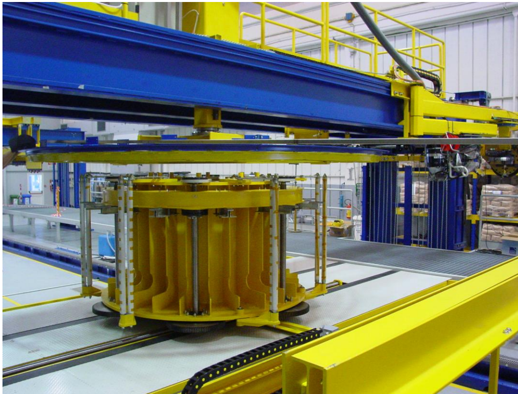
Figure 8 The de-spooling carriage is then moved underneath the reserve spool and it is laid down on top of the carriage.
