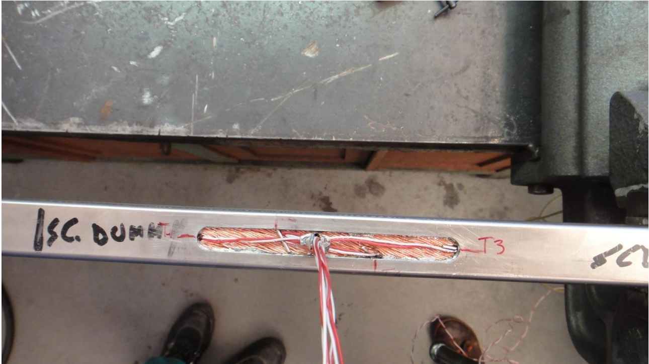
Fig. 2 Welding sample adopted to monitor the temperatures on the cable during welding
