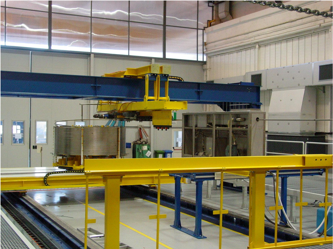
Figure 3 De-spooling, straightening and cleaning during reserve spool preparation
