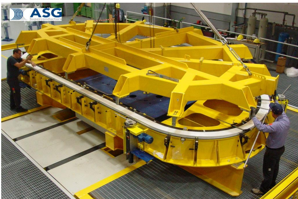
Figure 9 Lifting of using DP and WP lifting tool
