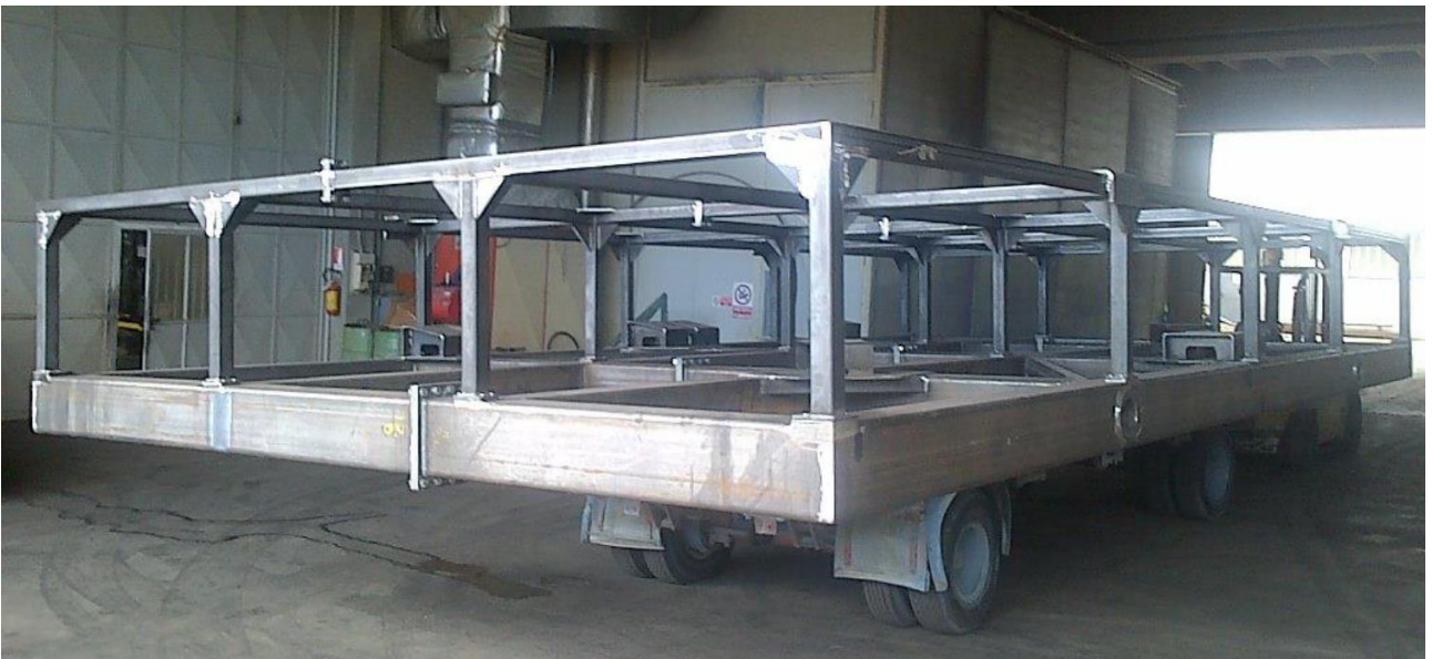
Figure 14 Present status of fabrication of the first transportation frame.
