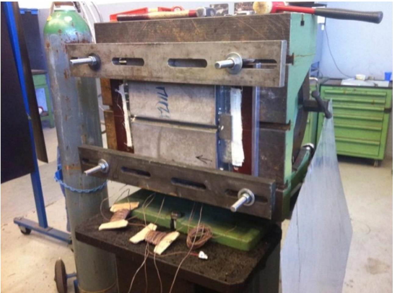
Figure 20 Transverse welding on 316L steel plates for chamfer confirmation and welding qualification
