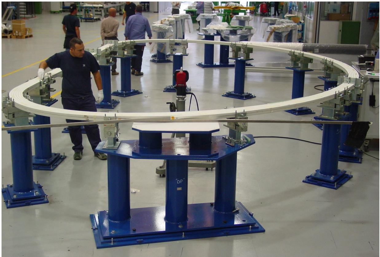
Figure 11 Dimensional survey on DP with laser tracker
