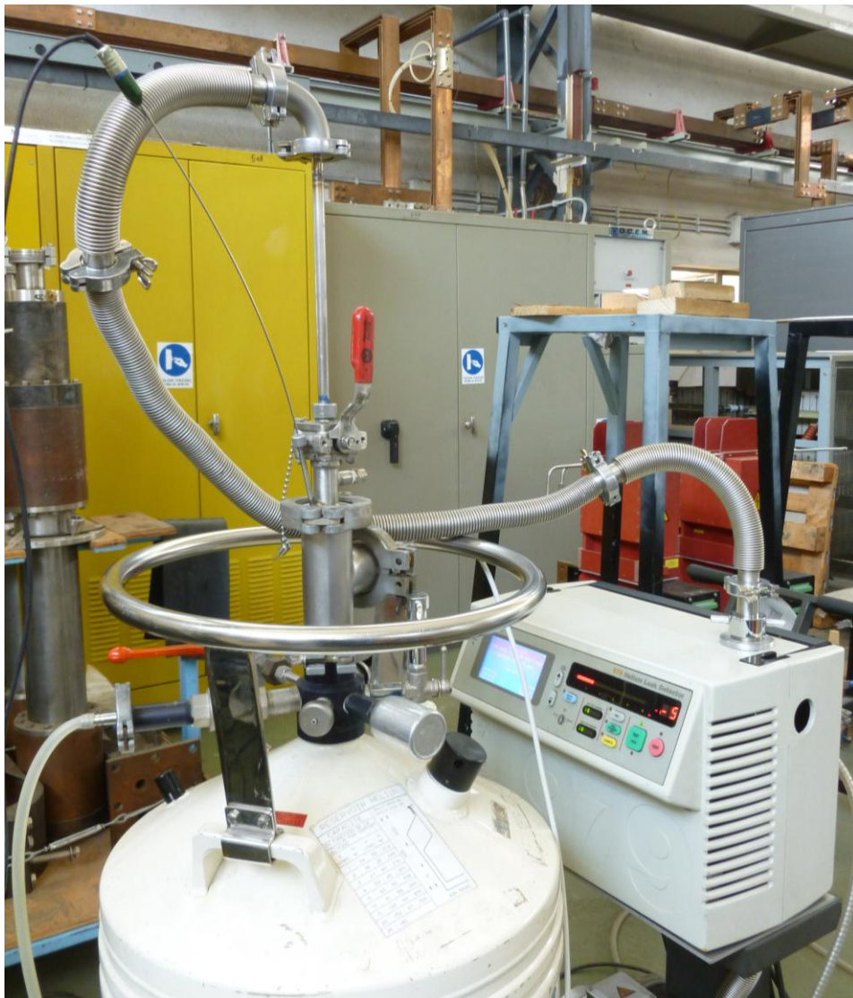
Figure 25 Facility set-up for electrical breaker leak testing in cryogenic conditions.
