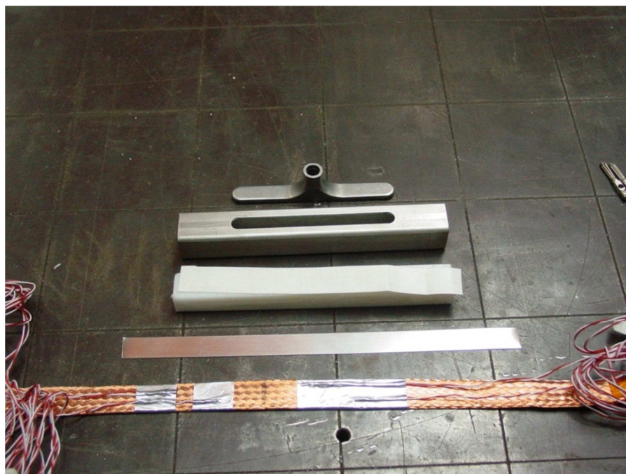
Fig.3 - Componenti per test preliminare: inserto ingresso He, tubo 25x25mm, riempitivo in nylon, lamierino sp=0.02mm, treccia in Cu con termocouple Components for preliminary test: He inlet, 25x25mm tube, filler, s.s. shim th=0.02mm, Cu cable with thermocouples
