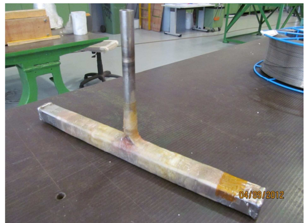
Fig. 12 – Campione He-inlet isolato / He-inlet insulation sample
