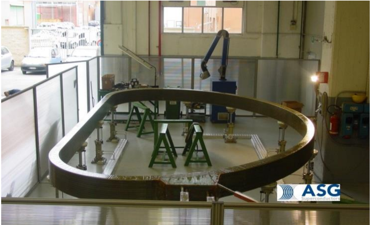
Fig. 12 WP01 on cleaning station before conductive paint is applied
