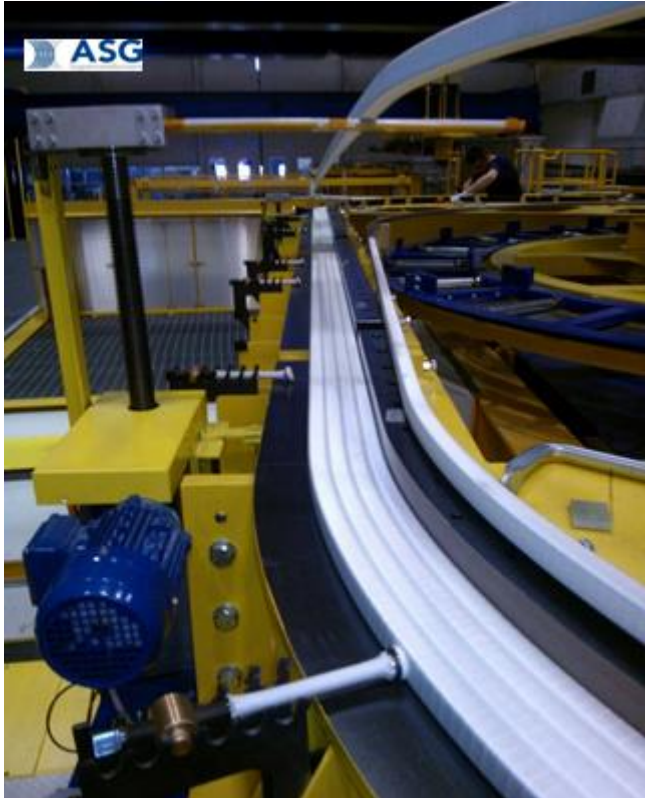
Fig. 2 -- Straight leg of the first pancake during winding onto the winding table
