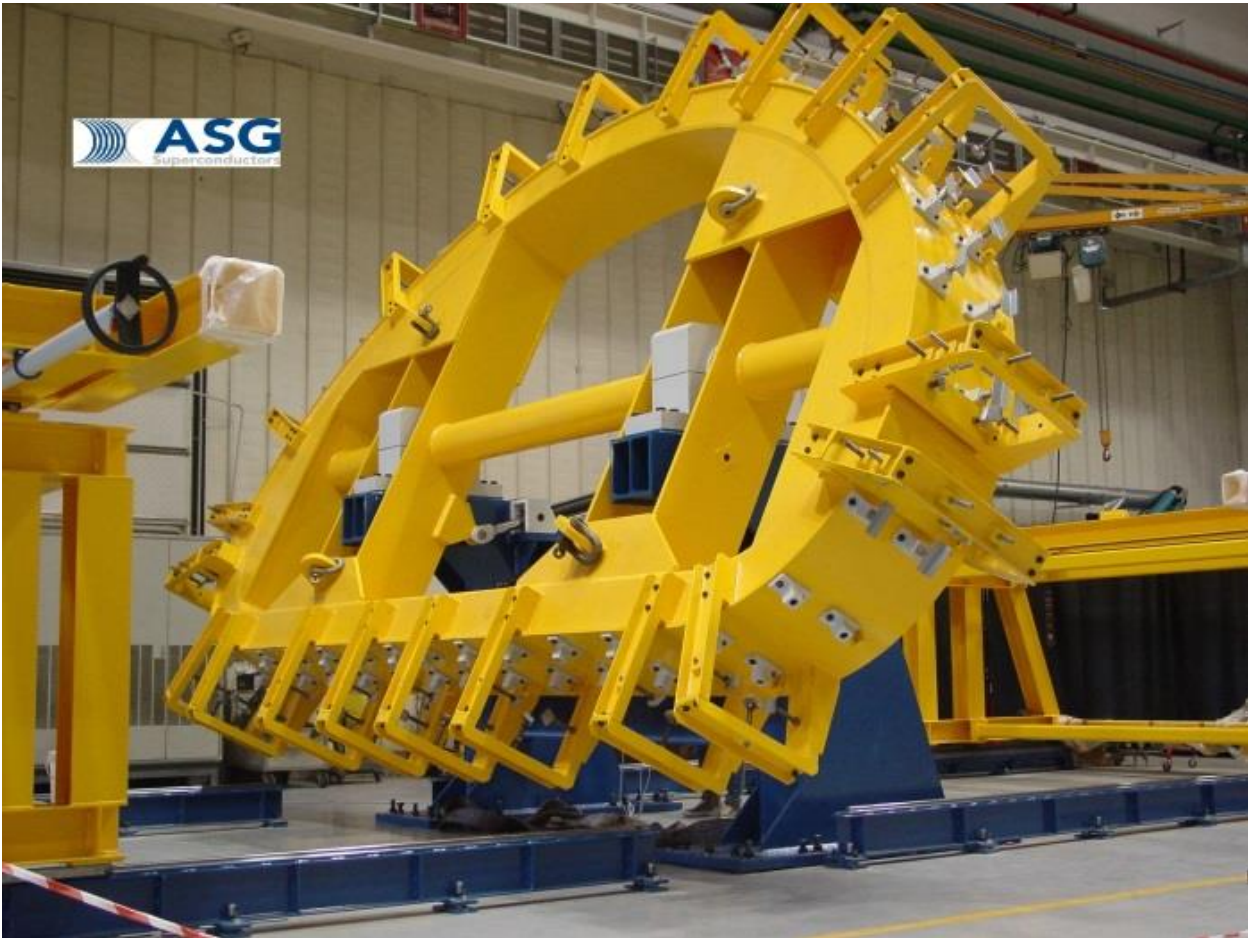
Fig.17 – Tooling for WP insertion into the casing.
