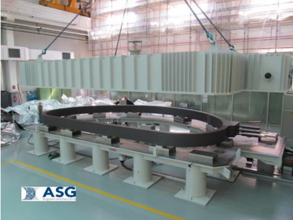
Fig.14 – WP01 inside D-shape vacuum tank at the completion of global leak test.
