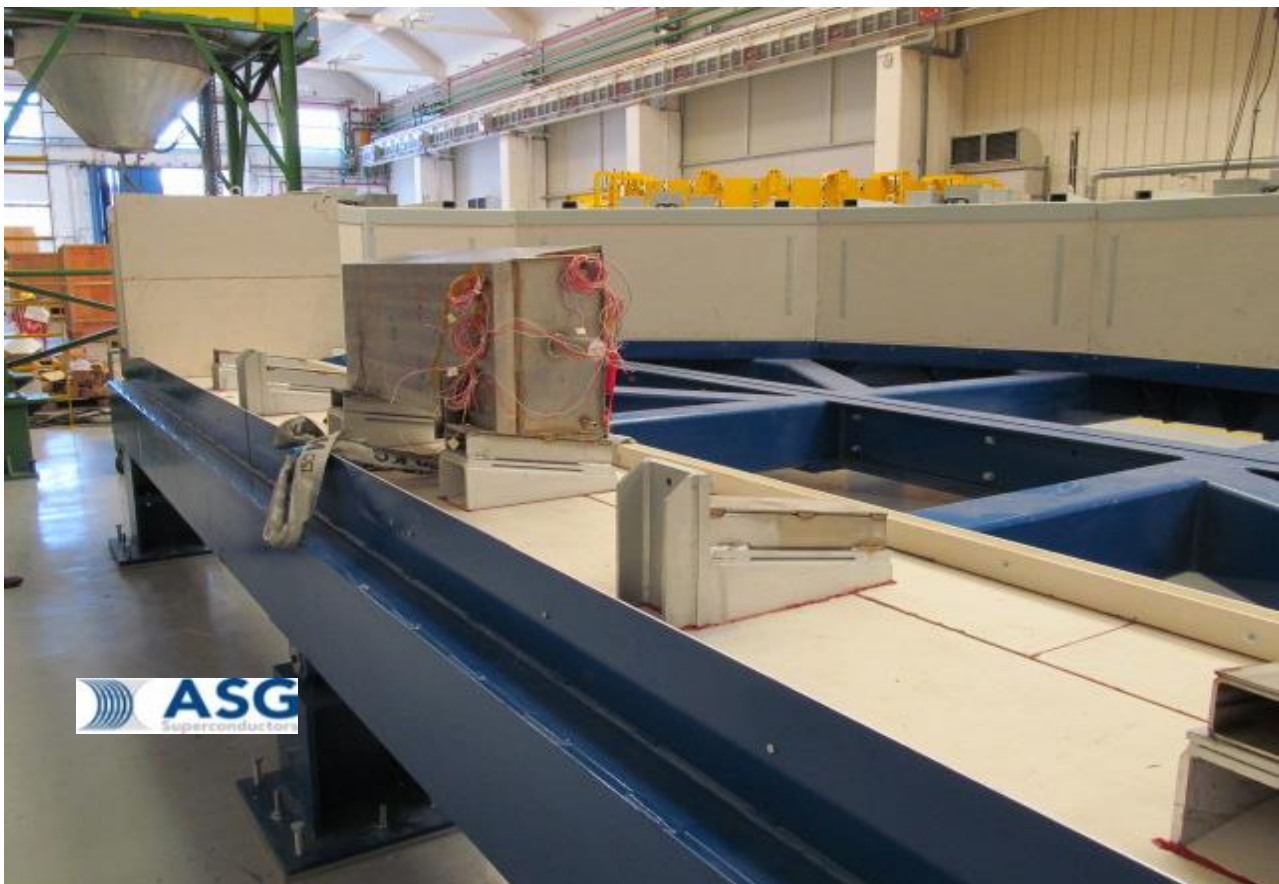
Fig.26 -- Straight leg mock-up ready for the final embedding.
