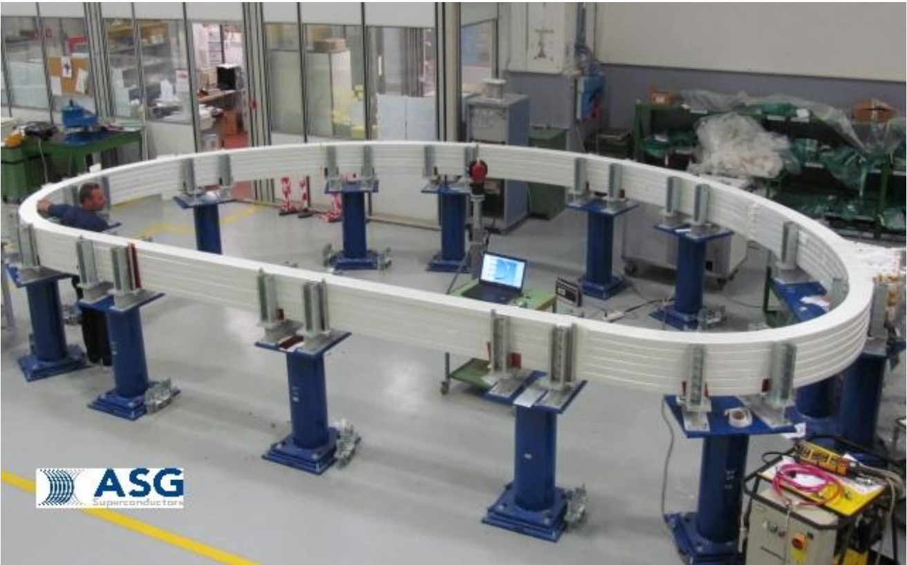
Fig.7 WP01 at the completion of stacking process
