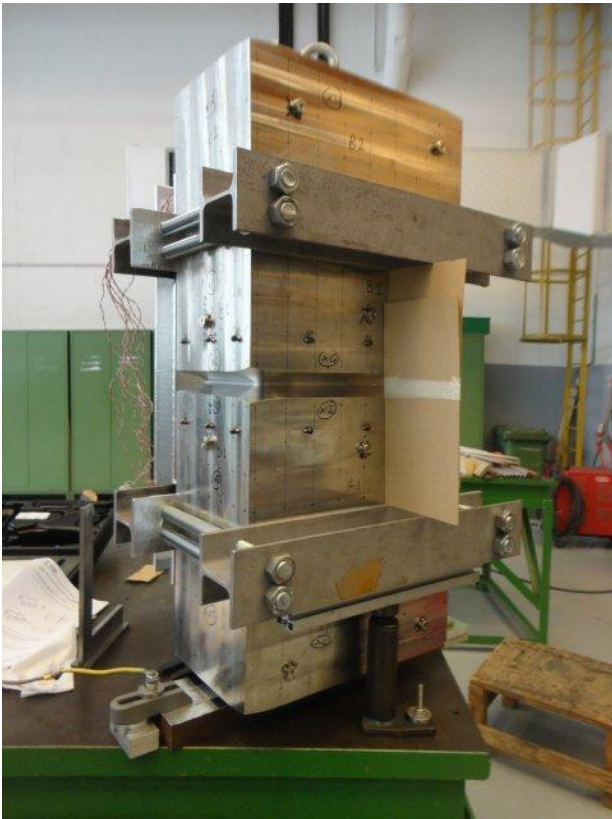
Fig. 24. Curved leg mock-up ready for transverse welding.
