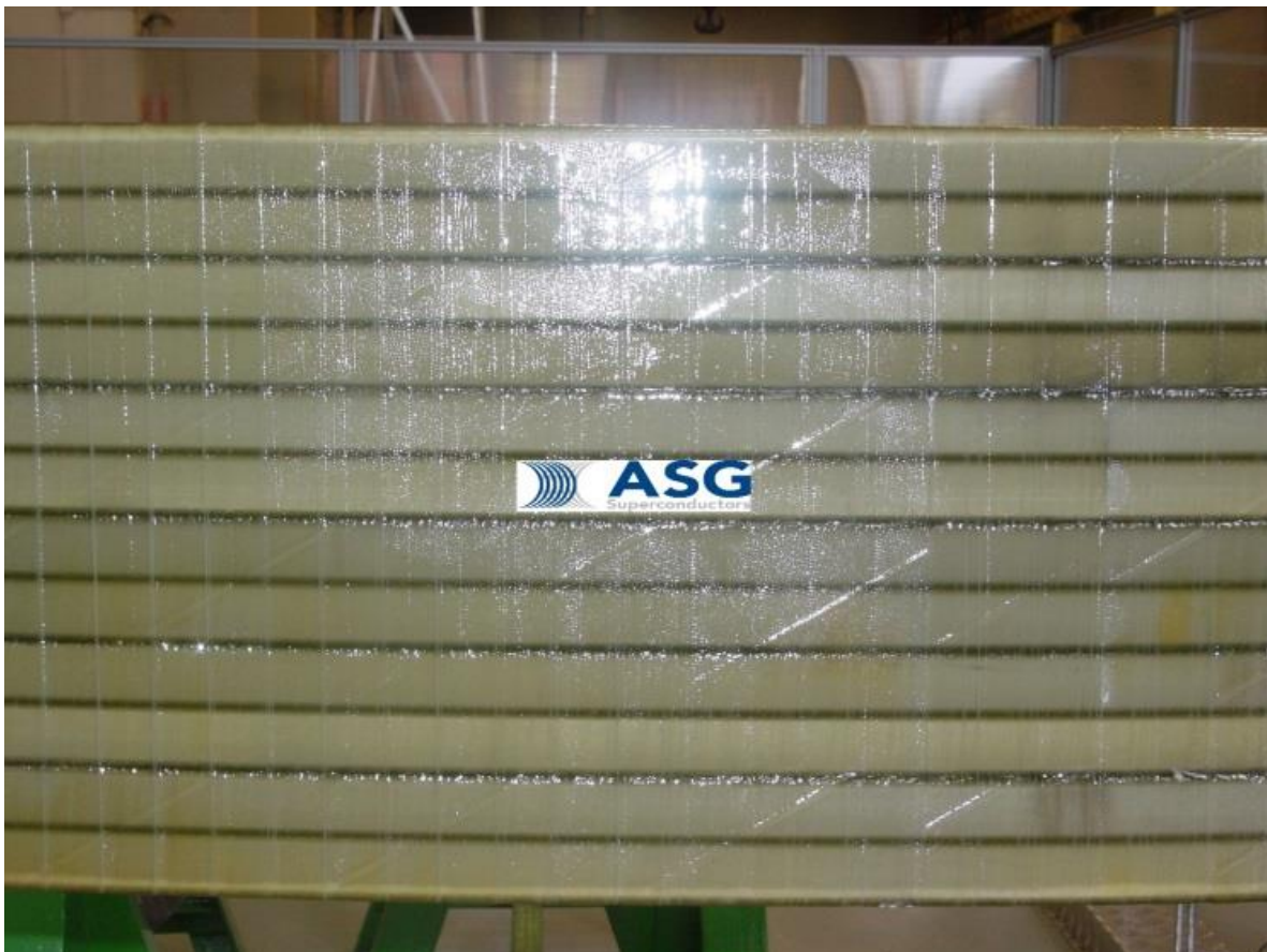
Fig. 13 – Visual inspection of WP01 impregnation
