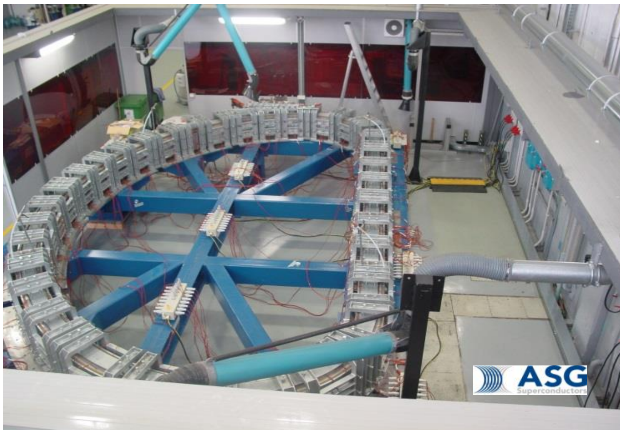
Fig. 10 WP01 at the beginning of the VPI process.
