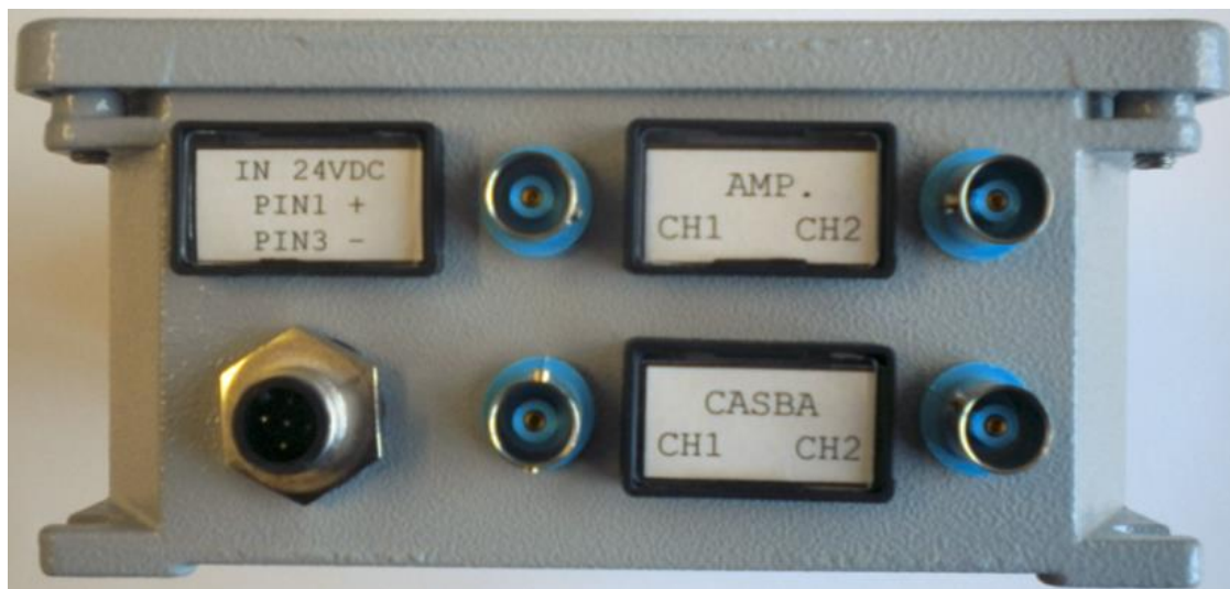
Fig. 5 Two channels power supply / signal splitter
