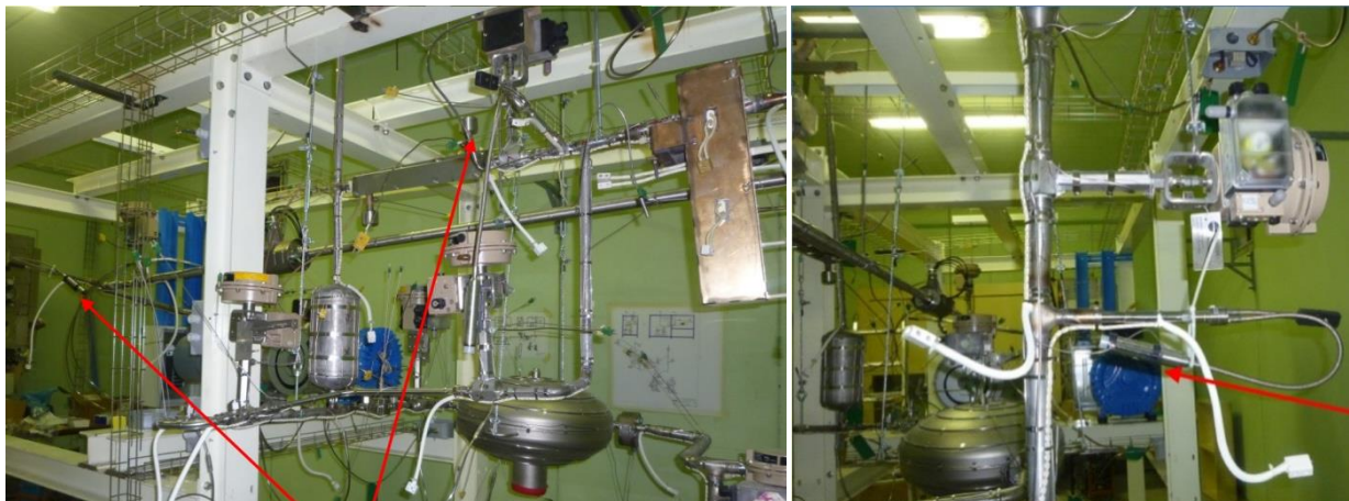
Figure 6: Pressure Transmitters. Left: EM pump outlet and purification line; right: Test Section outlet
