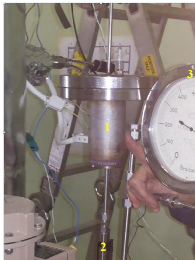
Figure 4: the sampler installed on the top of the Hot Trap. 1: sampler; 2: connecting pipe to the Hot Trap; 3: pressure gauge for the measurement of the pressure in the below Hot Trap
