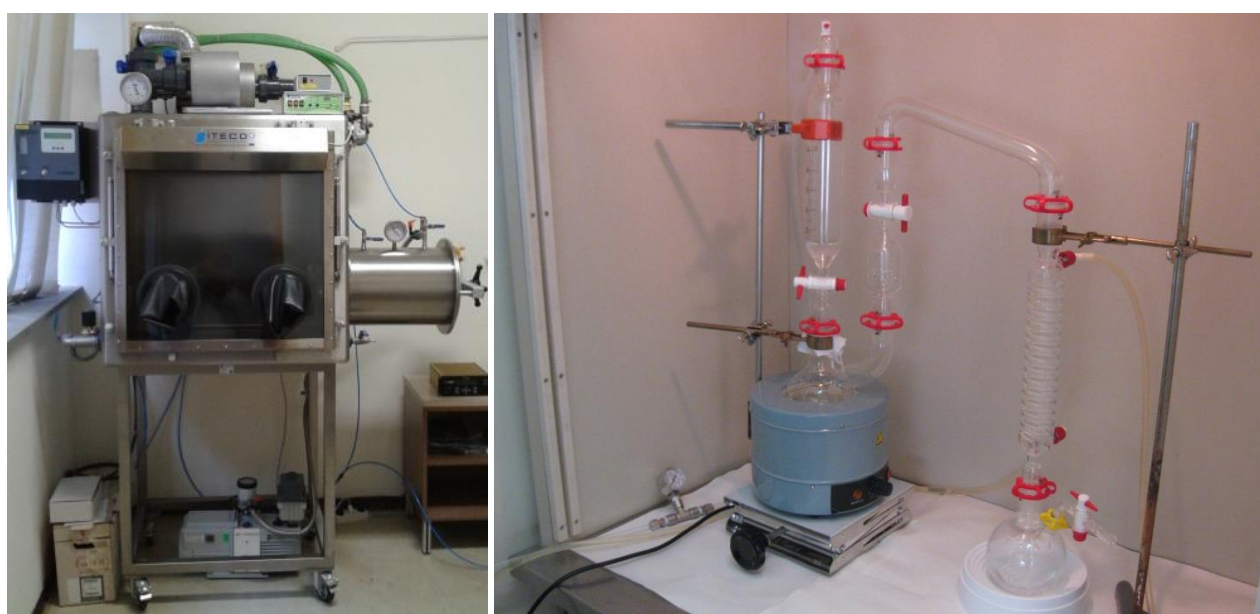
Figure 6: Equipment in Brasimone ENEA lab. Left: the new glovebox, employed for Lithium handling; right: apparatus for the Lithium-water reaction and the distillation of the produced Ammonia
