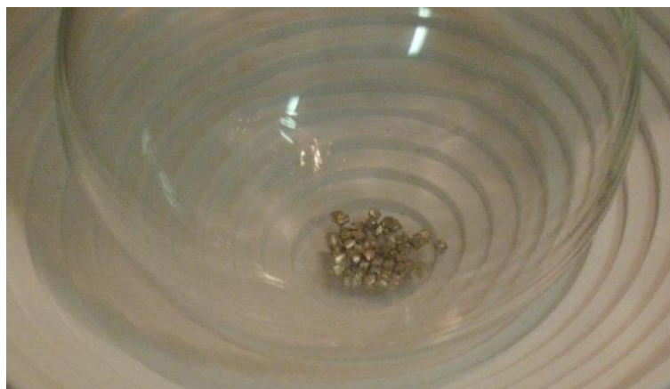
Figure 7: shining Lithium inside the main flask (in Argon atmosphere)
