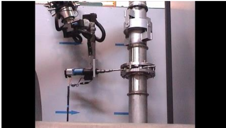
Fig. 25 Unlocking of the FDS in the inlet side
