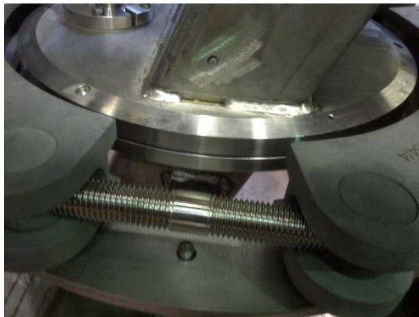
Fig. 24 Gap between the FDS' flanges on the outlet channel
