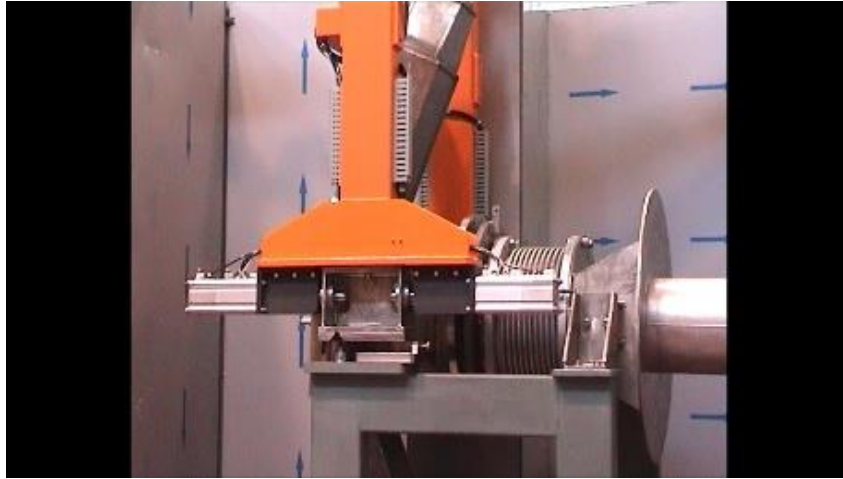
Fig. 28. Removal of the TA
