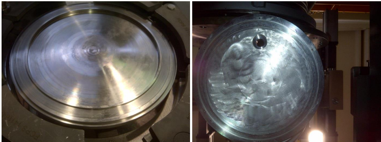
Fig. 31 Status of the flanges of the FDS on the outlet channel
