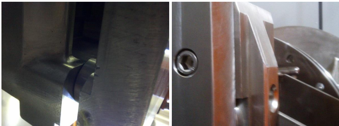
Fig. 20 Damages occurred in the lower side and in the guides of the BP
