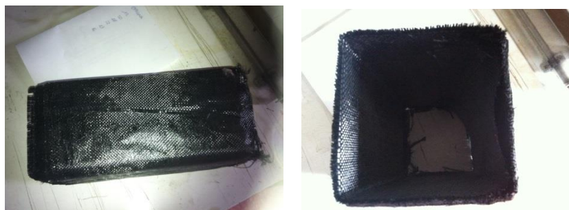
Figura 18. Preforma prisma in SiC/SiC
