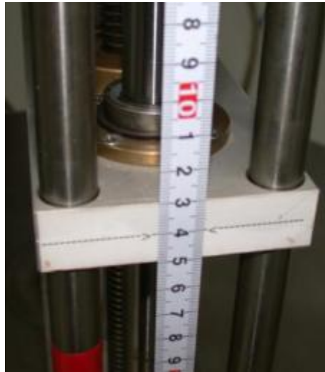
Figure 34: Manual translation system at 140 mm
