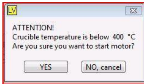
Figure 16: Warning window appearing if the electrical motor is actuated when the temperature of the crucible is below 400°C
