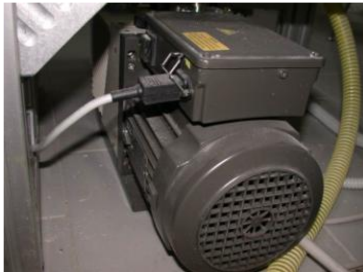
Figure 5: Vacuum pump electrical connections
