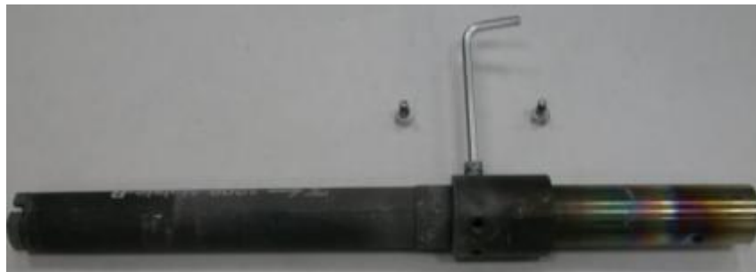
Figure 15: silicon carbide tube joined to the steel rotating tube
