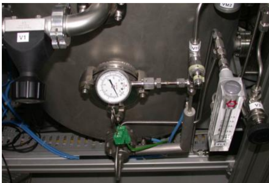
Figure 42a: Position of the argon system valves
