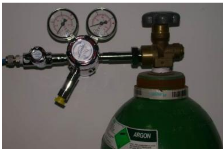
Figure 43: Establish a pressure in the argon line
