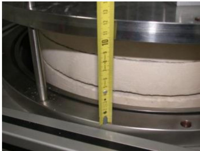
Figure 33: lowering of the closure flange at 100 mm
