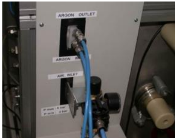
Figure 6: Inlet/outlet argon and inlet air pressure
