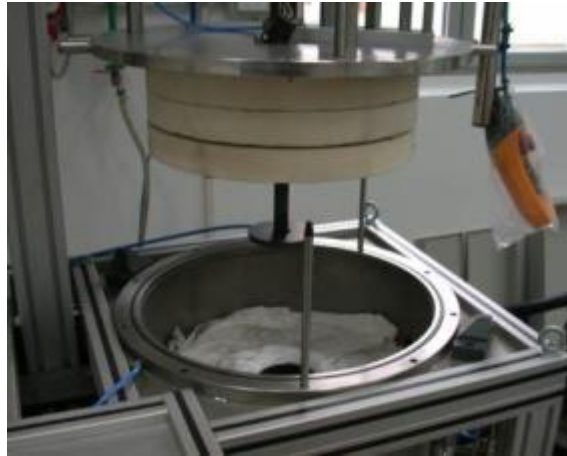
Figure 30: Positioning of the closure flange on the furnace
