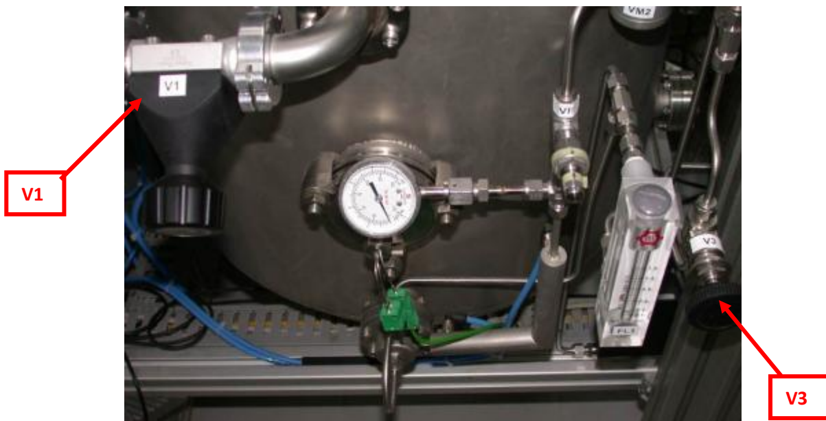
Figure 20: Position of the argon system valve
