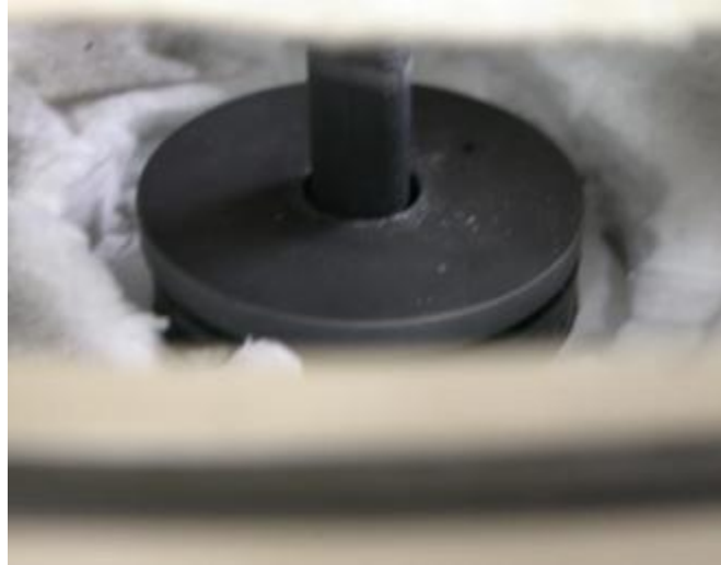
Figure 32: well-positioning of the cap over the crucible
