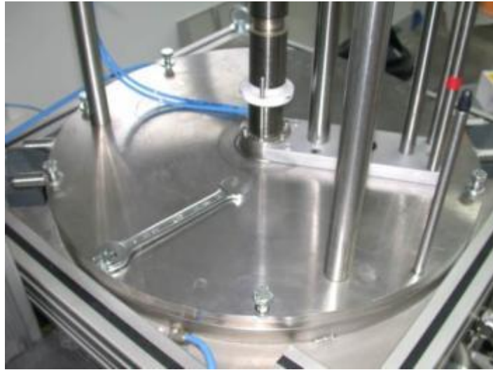
Figure 41: Fix the closure flange
