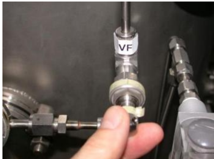
Figure 45: position of the manual regulator valve VF
