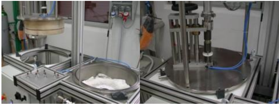
Figure 22: Positioning of the closure flange in the working area (on the left side of the furnace)
