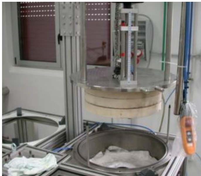
Figure 21: Lifting of the closure flange
