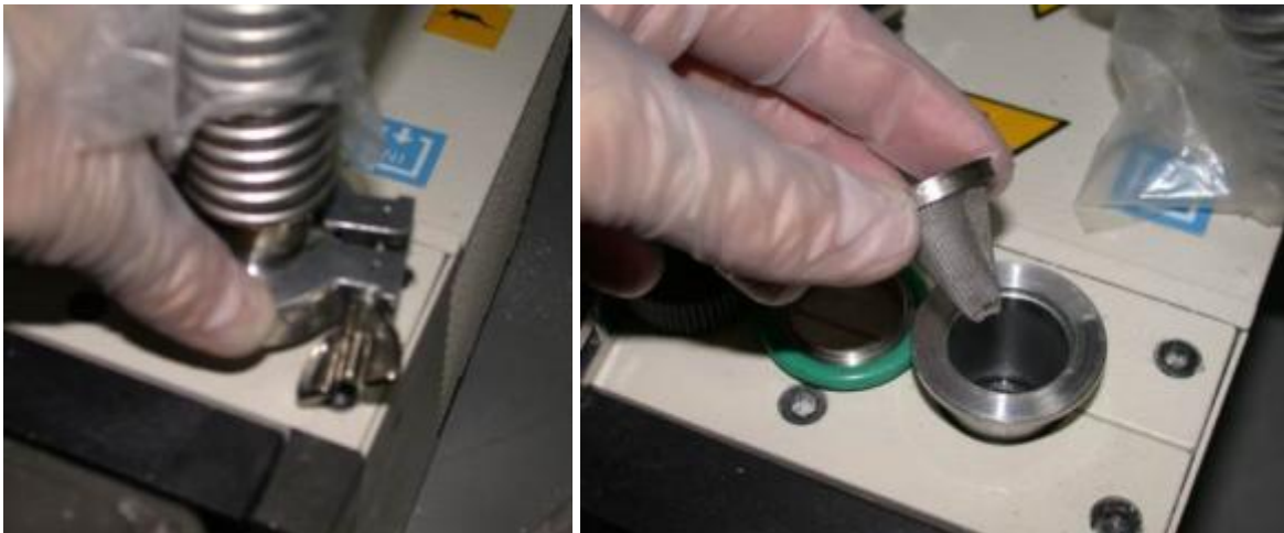
Figure 42: Cleaning of the vacuum pump filter
