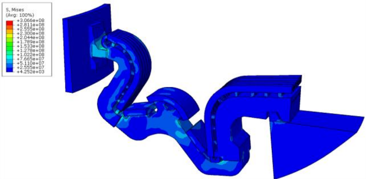
Fig. 25. Von Mises Stresses overview: time instant 67.9ms.
