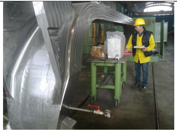
Figura 11: Pressure test e leak test.
