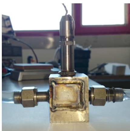
Figure 13: Flowmeter with welded cover sheet
