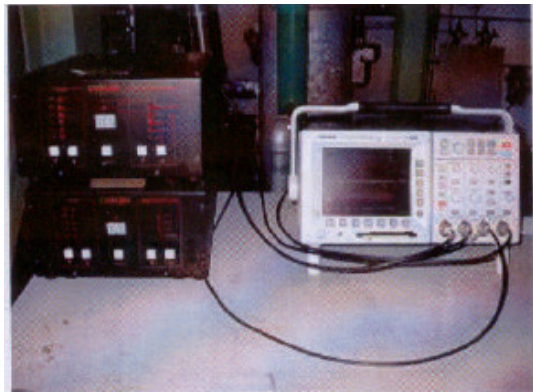
Figure 1: ENEA Cavitation detector equipment: a)-b) accelerometer transducer; c)-d) CASBA-2000 units and a digital oscilloscope
