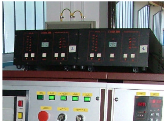
Figure 1: ENEA Cavitation detector equipment: a)-b) accelerometer transducer; c)-d) CASBA-2000 units and a digital oscilloscope
