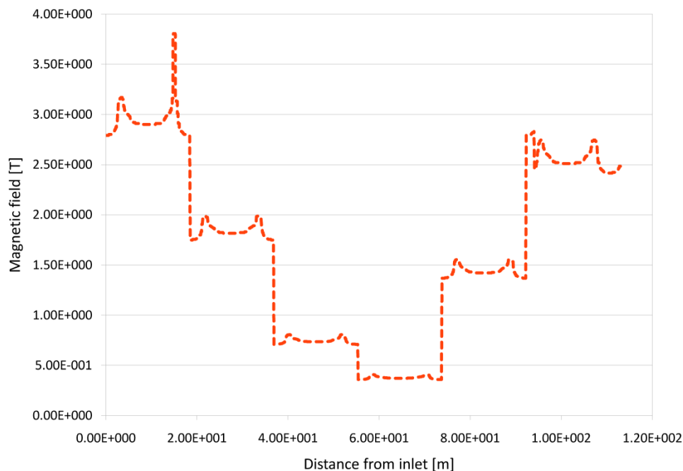
Figure 1 Distribution of magnetic field self-induced in the WP during cold test
