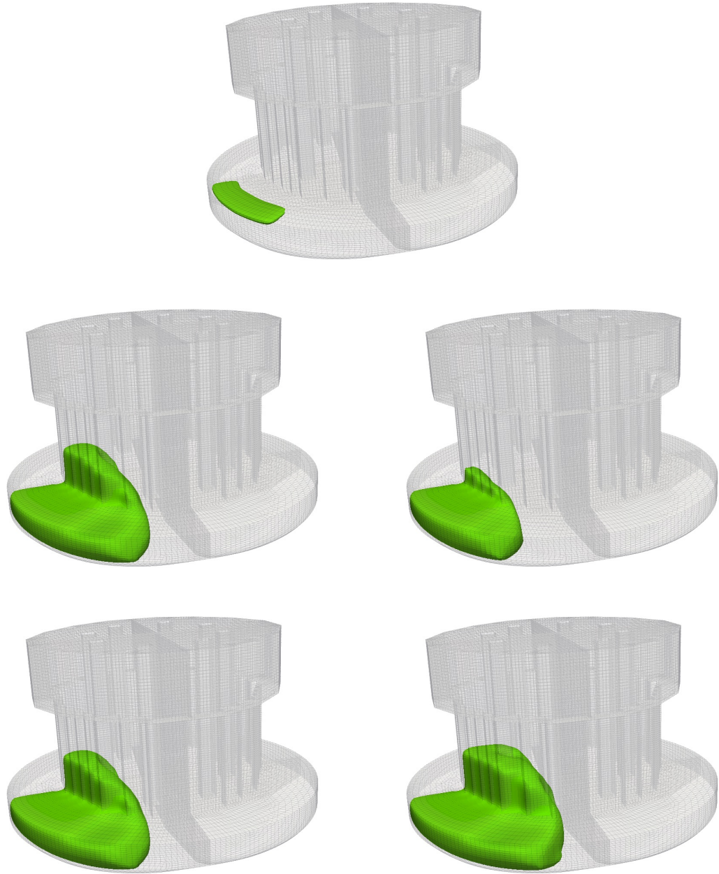
Figure 3.13: Test 4. Evolution of the freezing region for t = 0, t = 50, 100, 150 and 200s .
