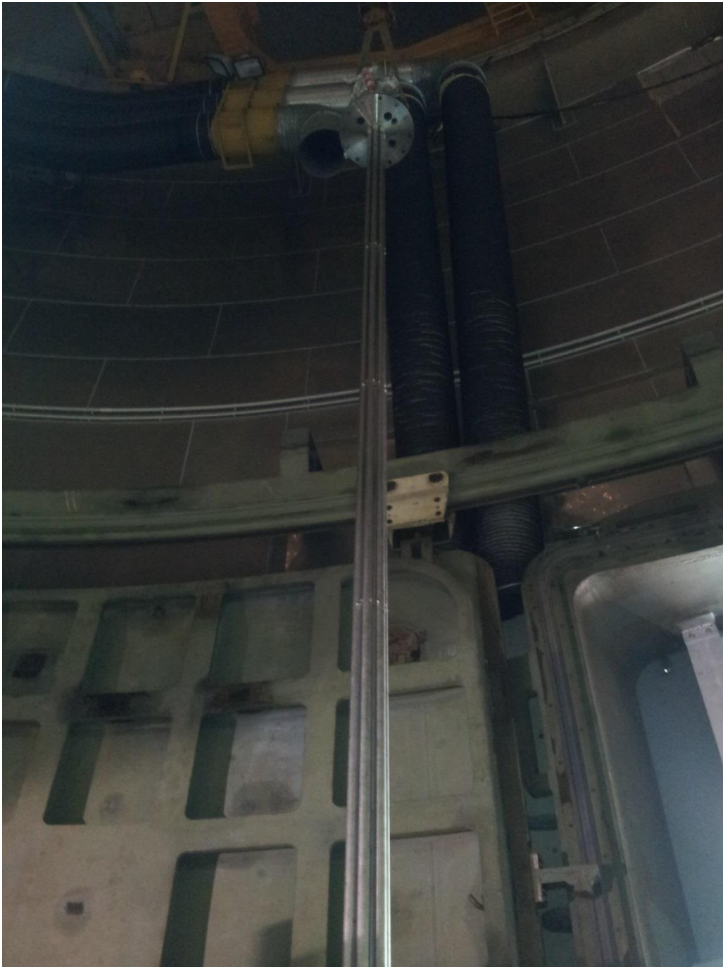
Figure 24 – HERO – CIRCE unit: bundle arrangement.
