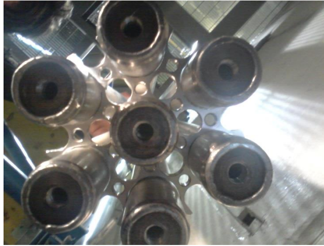
Figure 27 – HERO – CIRCE unit: end of bayonet tubes.
