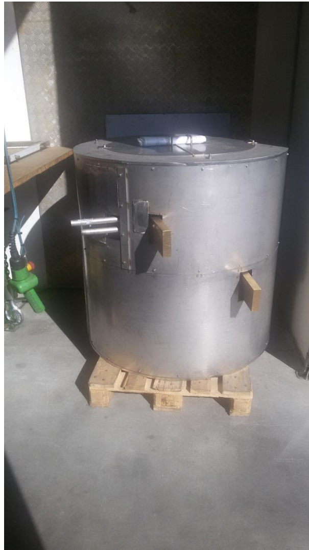
b) Spiral heater containment.
