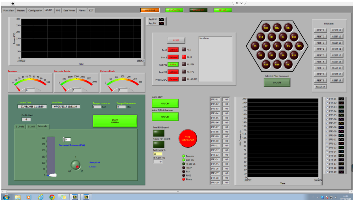
Figure.16: Control panel of the Fuel Pin simulator power
