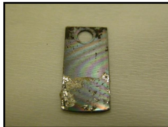
Coated samples by Al 2 O 3 (IIT)
