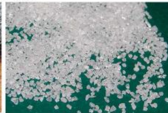
Fused corundum (screened size Al 2 O 3 ) Granular size - 0.8-1.2 mm, Heat resistance >1000°C
