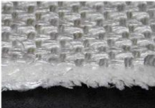
Fiber glass MKTT-2,2A SiO 2 >95 %, Fiber diameter ~ 6mkm, Heat resistance - 450°C
