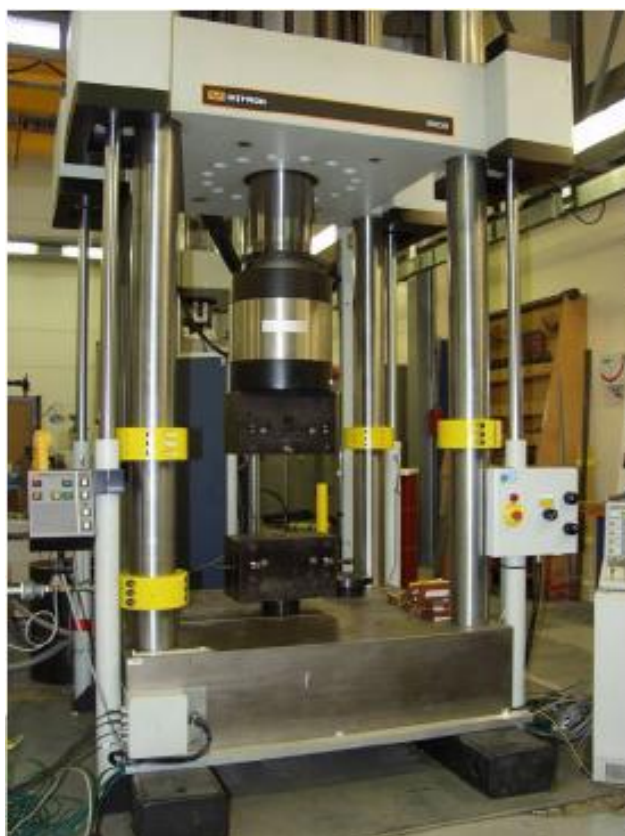
Fig. 4-4 – INSTRON 2500 kN tensile testing machine
