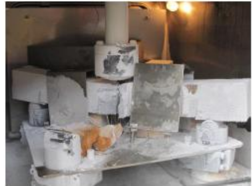
Fig. 4-11 – Specimen and bending device after the test
