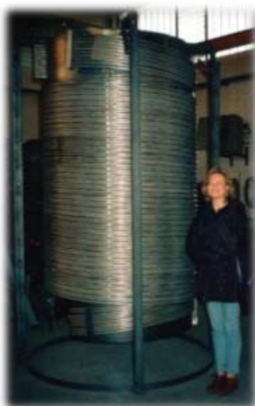
Prototypic 20 MW bundle, tested originally for ISIS Ansaldo reactor and having the same diameter as one of the IRIS Steam Generators
