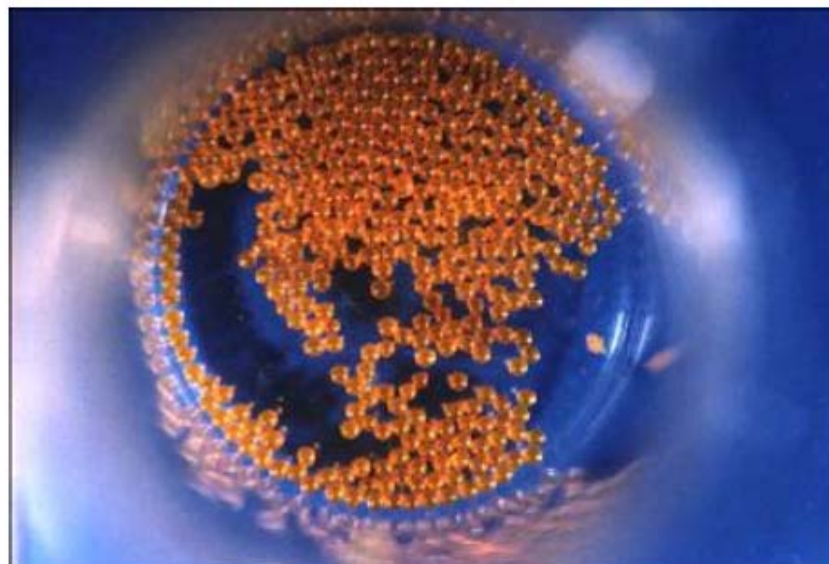
Figure 3.14.3 Fuel uranium kernel
