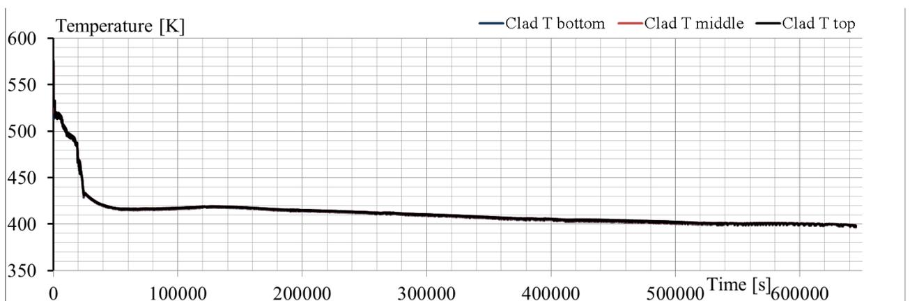
*Fig. 6.3 – Simulation of SBO transient: cladding temperature*
