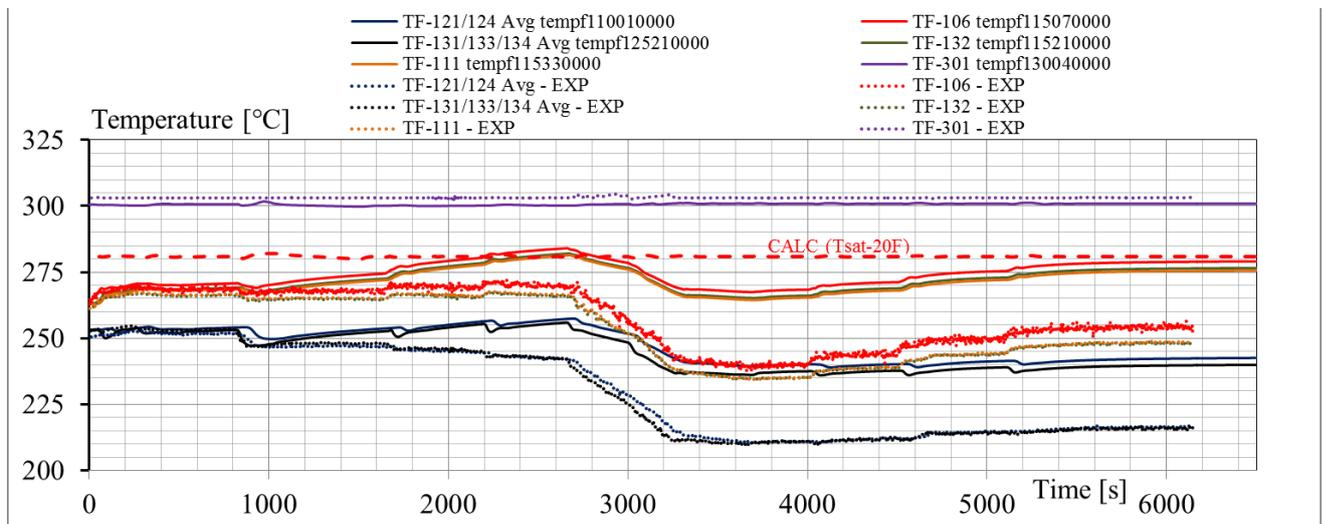
**Fig. 5.13 – Test SP3, blind pretest vs. experimental results: primary system coolant temperature, liquid phase (lower plenum, core outlet, SG outlet, riser, riser outlet and PRZ)**
