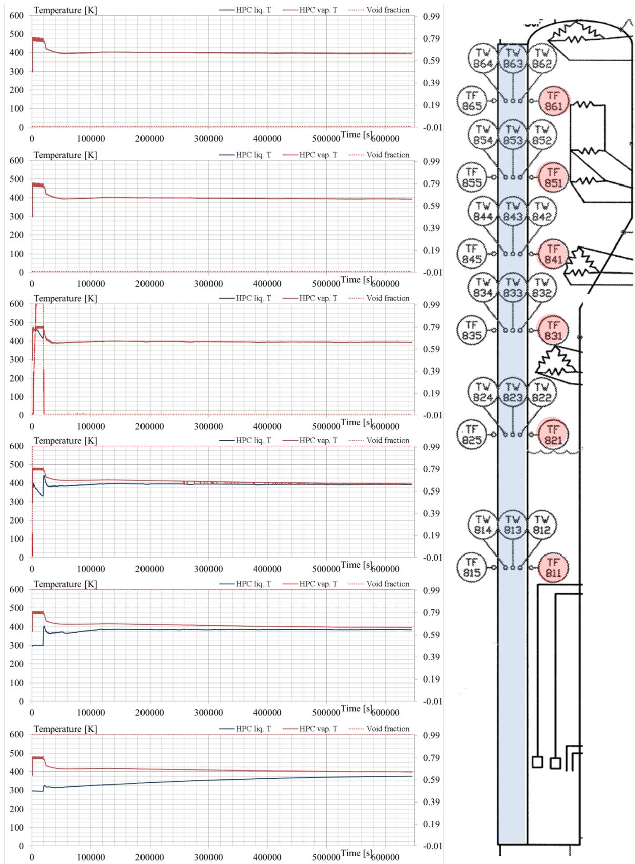
Fig. 6.9 – Simulation of SBO transient: HPC coolant temperatures
