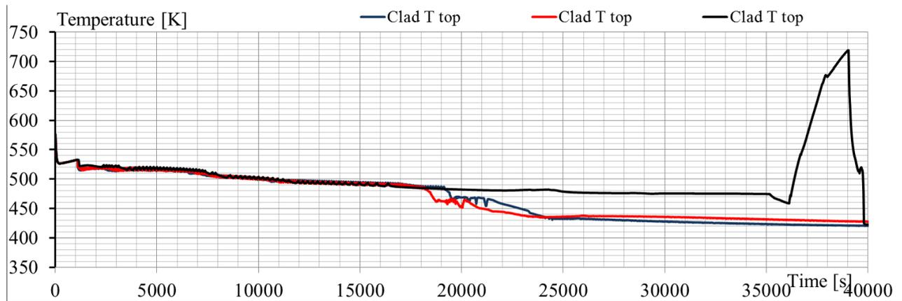
Fig. 6.15 – Sensitivity analysis RUN 1 vs. RUN 2 vs. RUN3: cladding temperature at top of the electrical core (blue “01a”; red “01a\_vlv05”, black “01a\_vlv01”)
