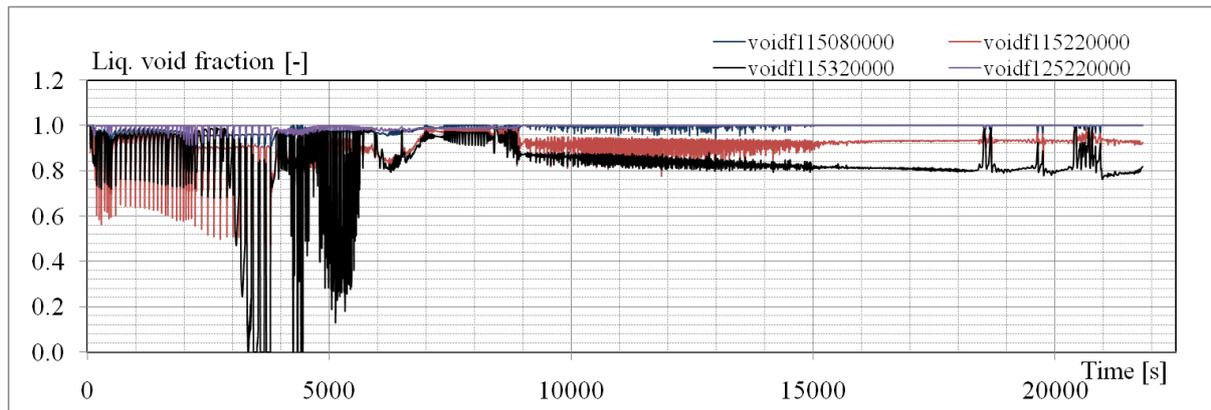
*Fig. 5.7 – Test SP2, blind pretest: liquid void fraction core outlet, riser bottom, riser top, SG outlet*
