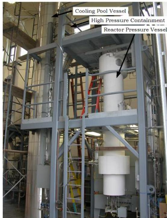
*Fig. 3.1 – Photo of OSU MASLWR Test Facility*
