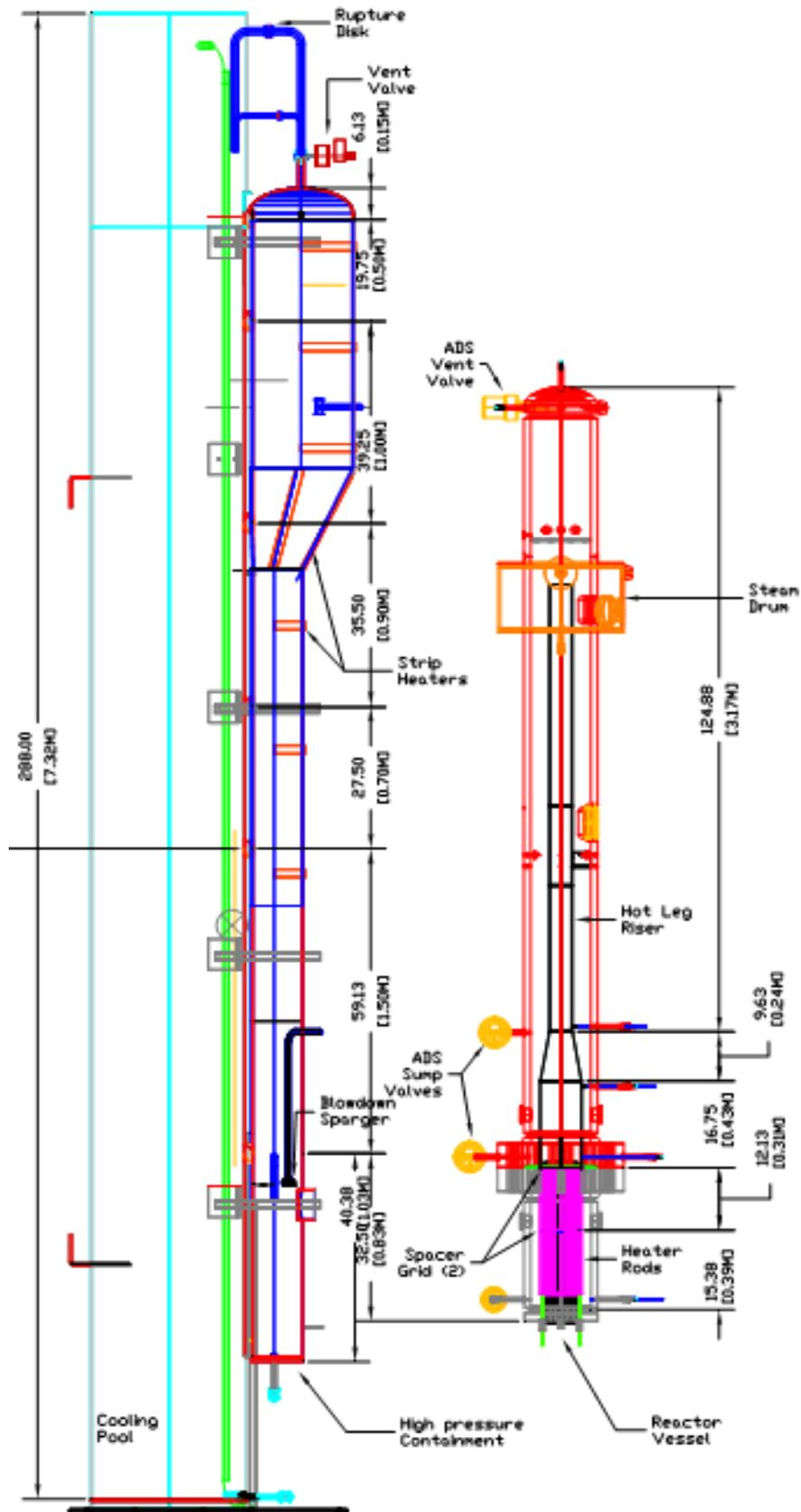
Fig. 3.3 – OSU MASLWR Test Facility: overall schematization
