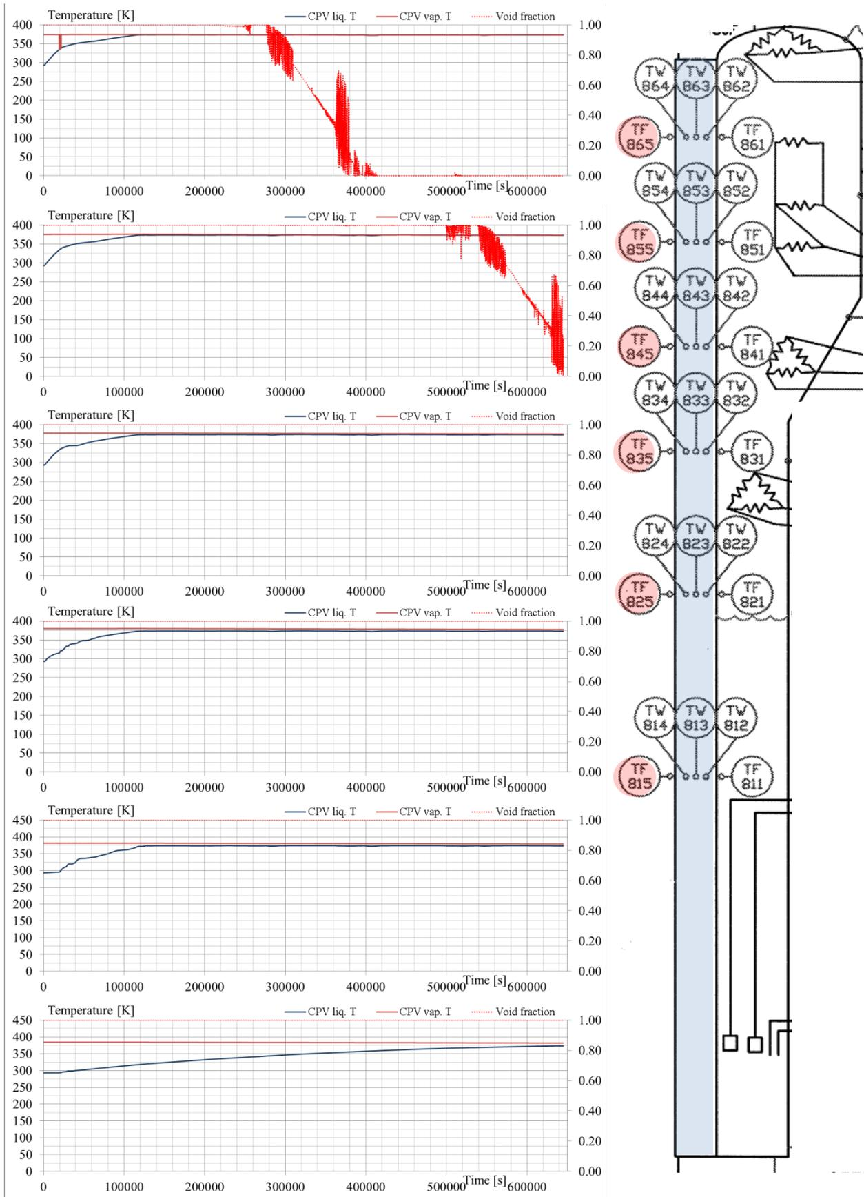
Fig. 6.10 – Simulation of SBO transient: CPV coolant temperatures
