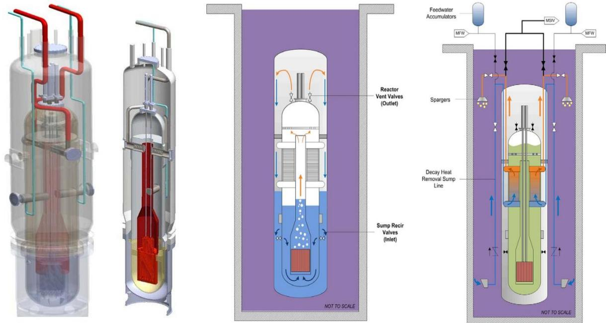
(a) High Pressure Containment Vessel and Reactor Pressure Vessel
