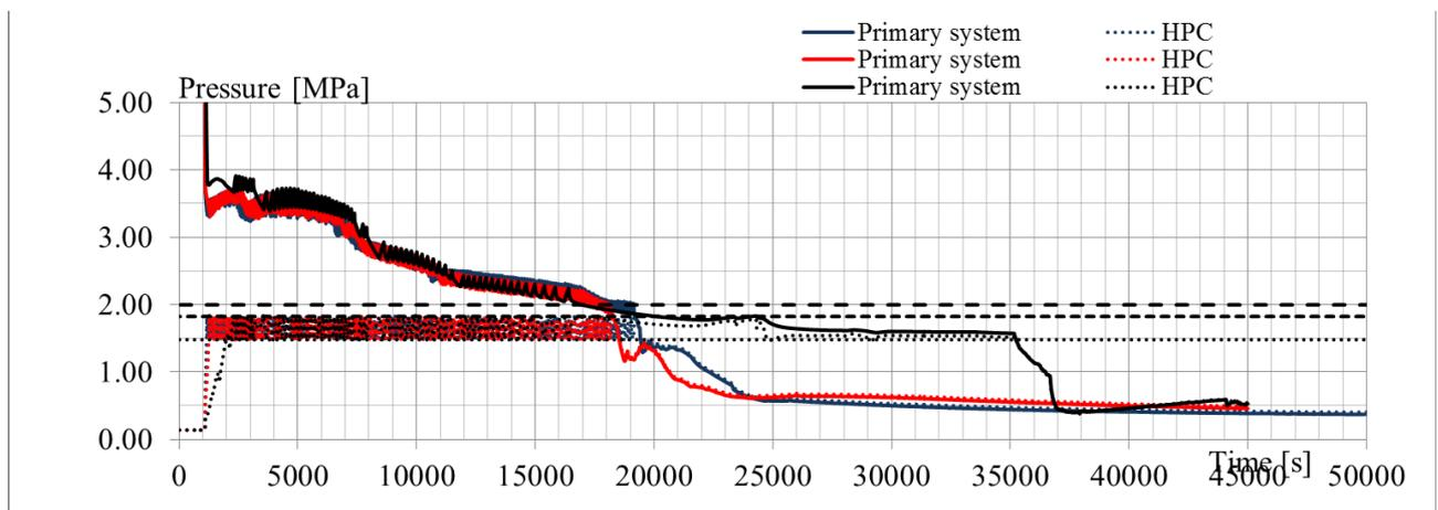
**Fig. 6.13 – Sensitivity analysis RUN 1 vs. RUN 2 vs. RUN3: primary system and HPC pressures (blue “01a”; red “01a\_vlv05”, black “01a\_vlv01”)**
