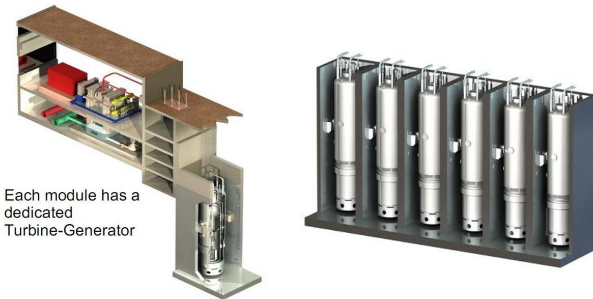
*(a) Schematic of the MASLWR exterior cooling pool and turbine generator set*
