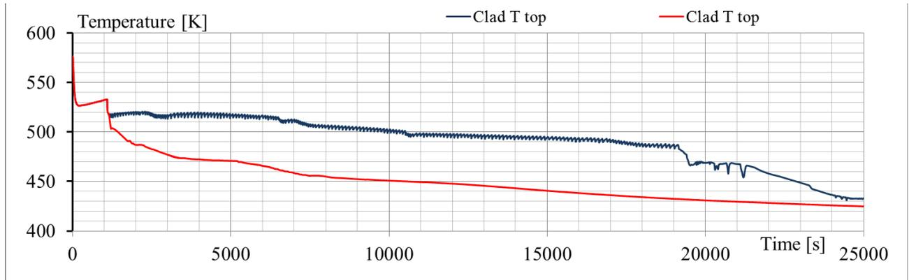
**Fig. 6.22 – Sensitivity analysis RUN 1 vs. RUN 6: cladding temperature at top of the electrical core (blue “01a”; red “03a”)**
