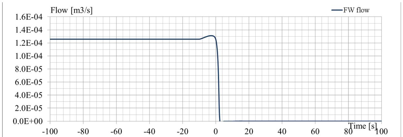
*Fig. 6.1 – Simulation of SBO transient: main FW flow*
