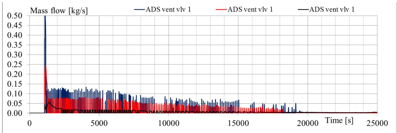
**Fig. 6.12 – Sensitivity analysis RUN 1 vs. RUN 2 vs. RUN3: ADS vent valve 1 mass flow rate (blue “01a”; red “01a\_vlv05”, black “01a\_vlv01”)**
