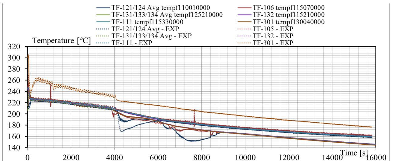
**Fig. 5.3 – Test SP2, blind pretest vs. experimental results: primary system coolant temperatures, liquid phase (lower plenum, core outlet, SG outlet, riser, riser outlet and PRZ)**
