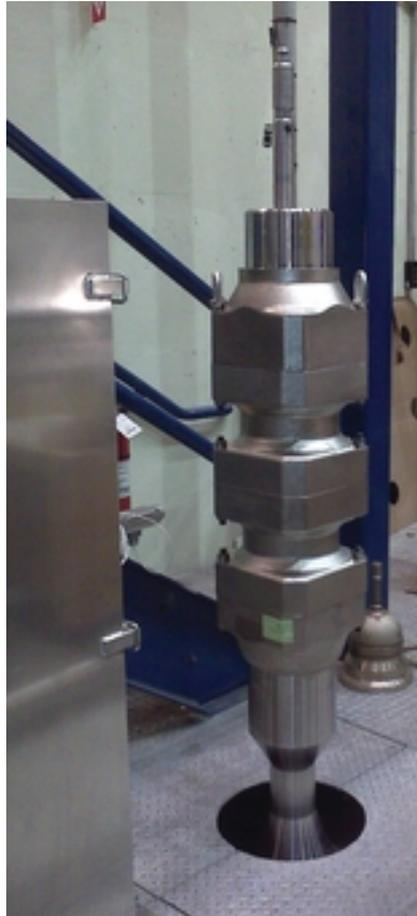
**Figura 4. CRDM: Control Rod Drive Mechanism (in prova)**
