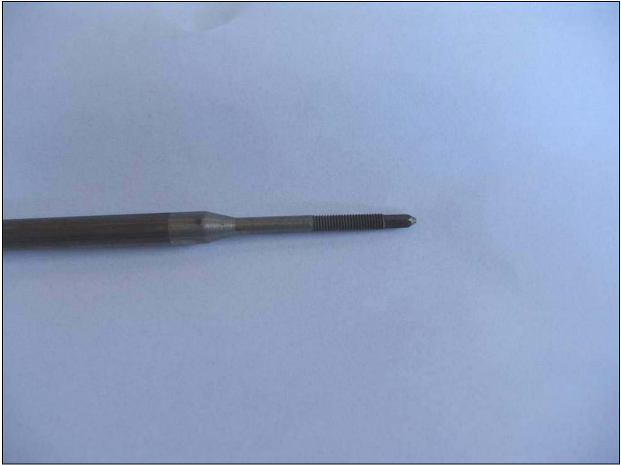
Fig.5. 2 – SPES-2 heater rod upper termination
