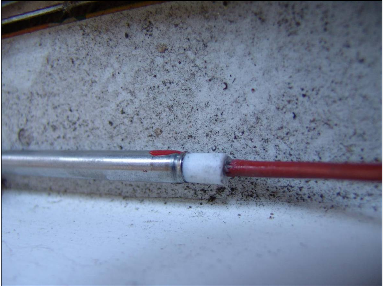
Fig.5. 1 – SPES-2 heater rod lower termination
