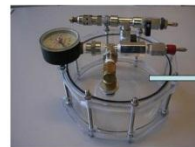
Cylindrical plexiglass container equipped by two valves for the vacuum pumping and the transfer of the gaseous sample
