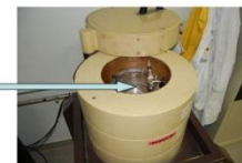
Positioning of the box in the well of the germanium detectors
