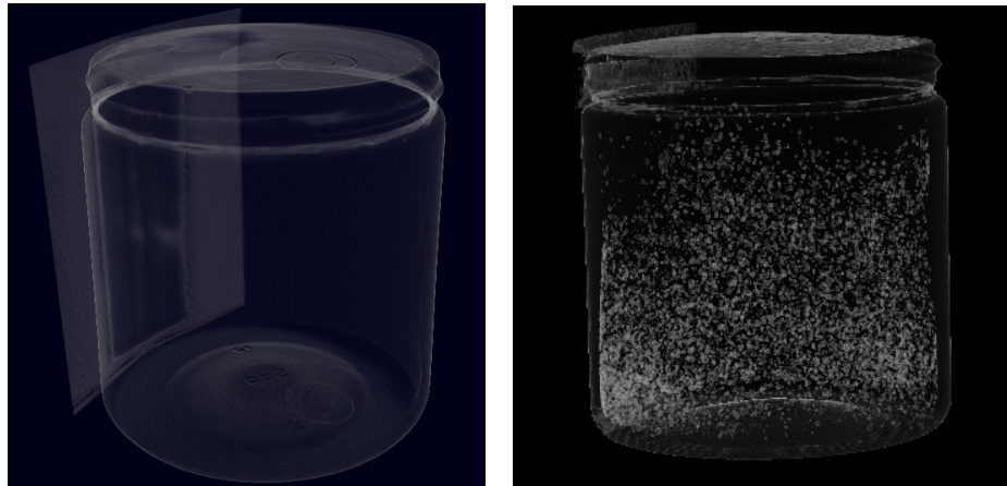
Figure A1. Computed tomography scans of a superheated emulsion of C-318 after an irradiation with 1 gray of 6 MV X-rays (left) and after an irradiation with 2.5 mSv of Am-Be neutrons (right) . The neutron irradiation was delivered using two sources in contact with opposite sides of the detector.
