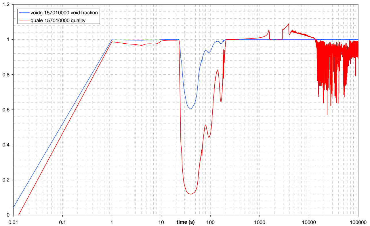
Figure 5.71: ADS ST SPLIT BREAK LINE void fraction and quality UPSTREAM
