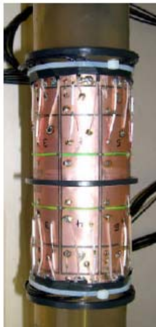
Fig. 101: ECT sensor mounted on transparent plastic pipe with electrical guard removed for clarity. (Azzopardi et al. (2010))
