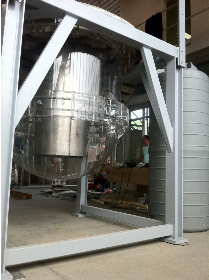
Figure 5. Photos of the lateral side of test section with the vessel containing water for the two DVI pipes
