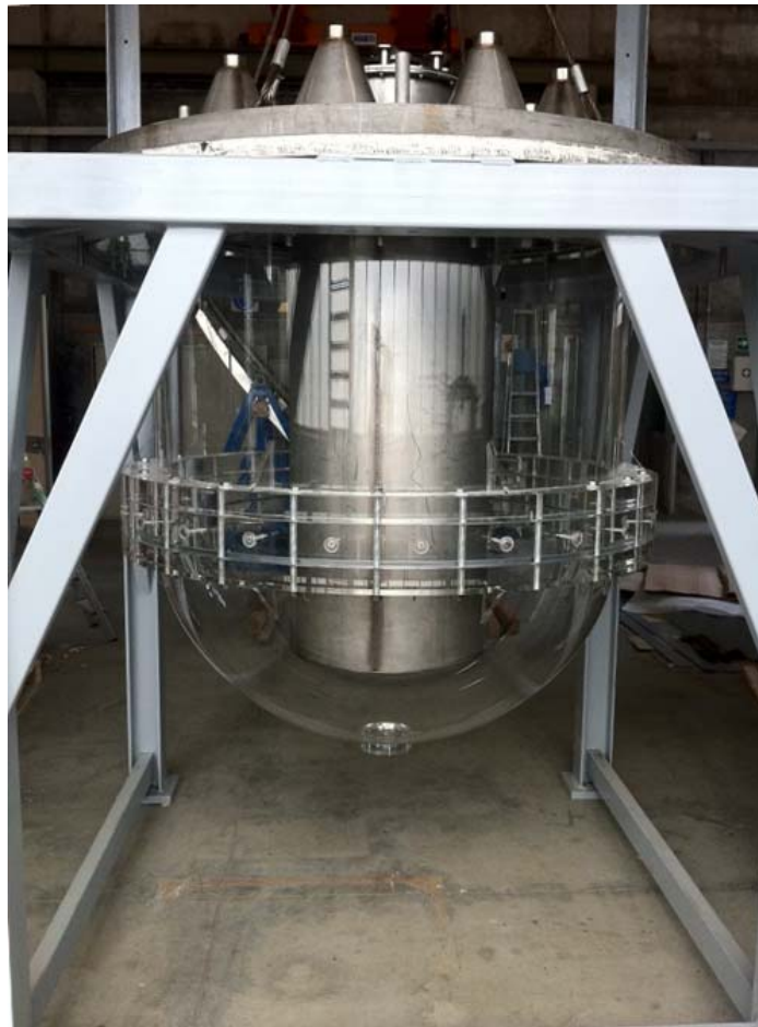
Figure 4. Photos of the lateral side of test section with support frame
